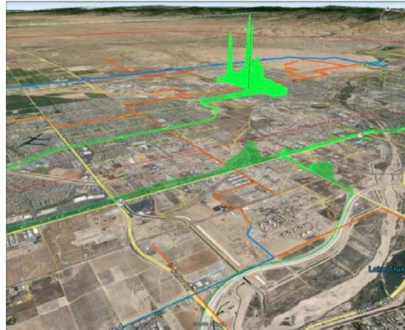
Methane above ambient (green), distribution (orange) and transmission (blue) pipelines
