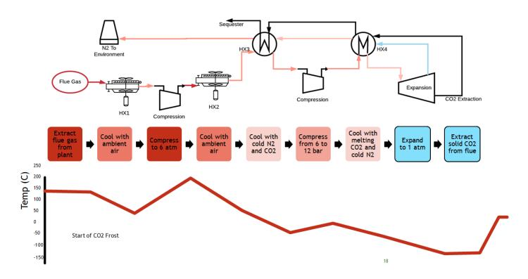
The diagram above illustrates how the cold nitrogen (all non-CO2 flue gases actually) that emerge downstream of the CO2 frosting process is recovered or recuperated making the energy required to run the process very competitive with other capture processes. Several key advantages include
