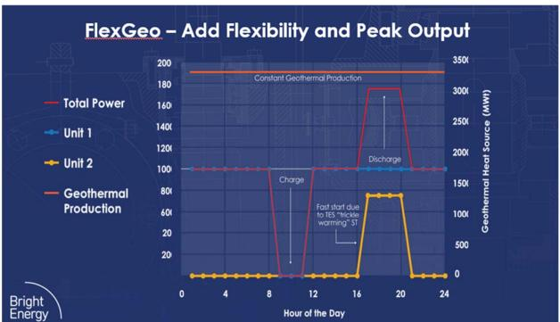
The addition of the CTES system allows the geothermal system to operate in accordance with the needed output to match the net generation requirements after the contributions from solar (the "duck curve"). This benefits the California grid by providing more carbon free peak capacity to meet resource requirements and benefits the economic viability of geothermal systems by providing for the sale of energy when prices are higher and also providing higher resource adequacy payments.
