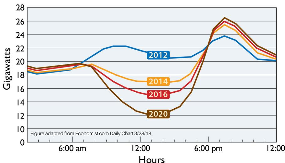
One of renewable energy's greatest challenges, the California "duck curve," shows the increasing daily supply of renewables over the years creates an increasing need for ramping conventional electricity starting around 4:00 PM each day.
