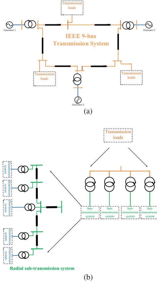
Fig. 4: Grid infrastructure to support DWPT systems in Scenario-1: (a) Transmission system, and (b) Sub-transmission system.
