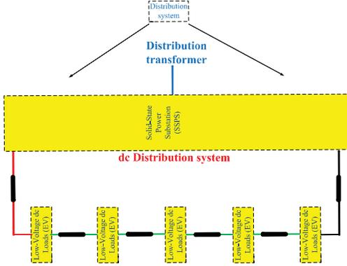
Fig. 7: The dc distribution system connected to the distribution transformer through solid-state power substation in Scenario-3.
