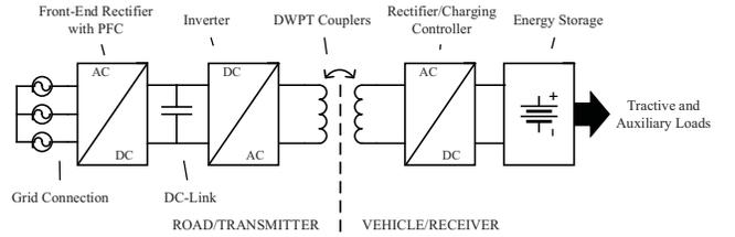
Fig. 2: DWPT system with active front-end (AFE) rectifier.
