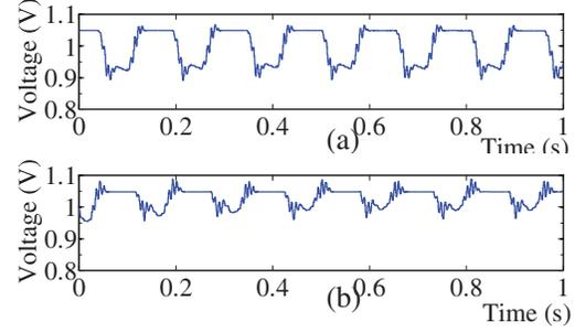
Fig. 8: Normalized voltage in a sub-transmission bus in Scenario-1: (a) Without smart inverters, and (b) With smart inverters.
