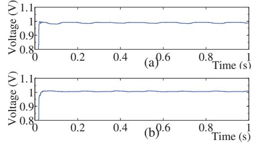
Fig. 9: Normalized voltage in a sub-transmission bus in Scenario-2: (a) Without smart inverters, and (b) With smart inverters.
