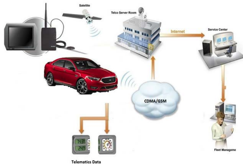
Image credit: Haulage Report Now Figure 1. Typical Telematics System
