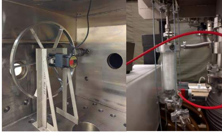
Figure I.12.3 - Rotating-wheel deposition system and the aerosol generator used to make long-length PLZT tapes.
