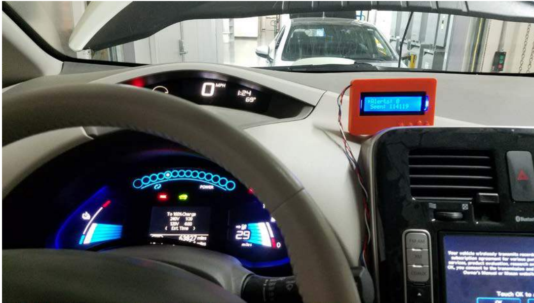
Figure IV.4.3 - DSM Installed in Nissan Leaf – Showing Status
