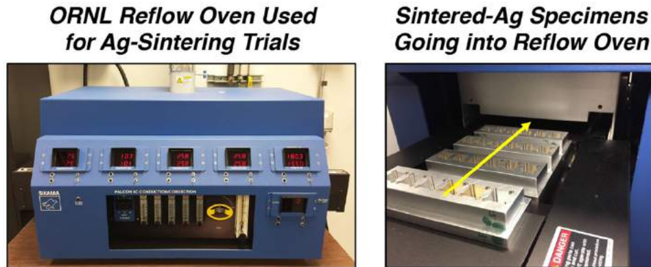
Figure I.8.4 - Reflow-oven processing is being used to sinter 200°C-capable Ag interconnects for PE devices.
