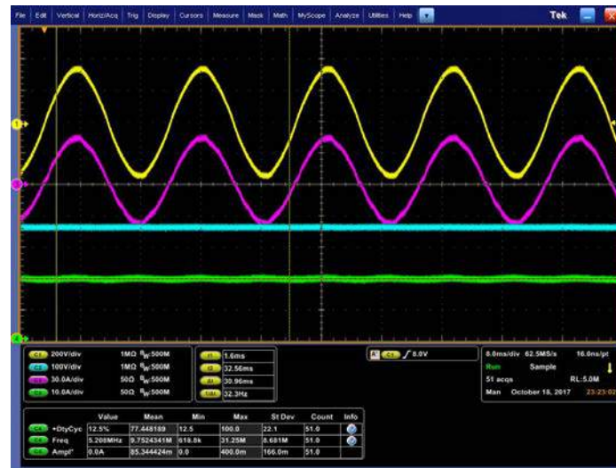
Figure II.1.2 - Level 2 charge waveform, Vout=350Vdc (CH1: Vac, CH2:Vdc, CH3:Iac, CH4:Idc)
