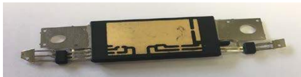
Figure II.6.2 - 650V, 1.7mΩ, SiC MOSFET Power Module Delphi Technologies
