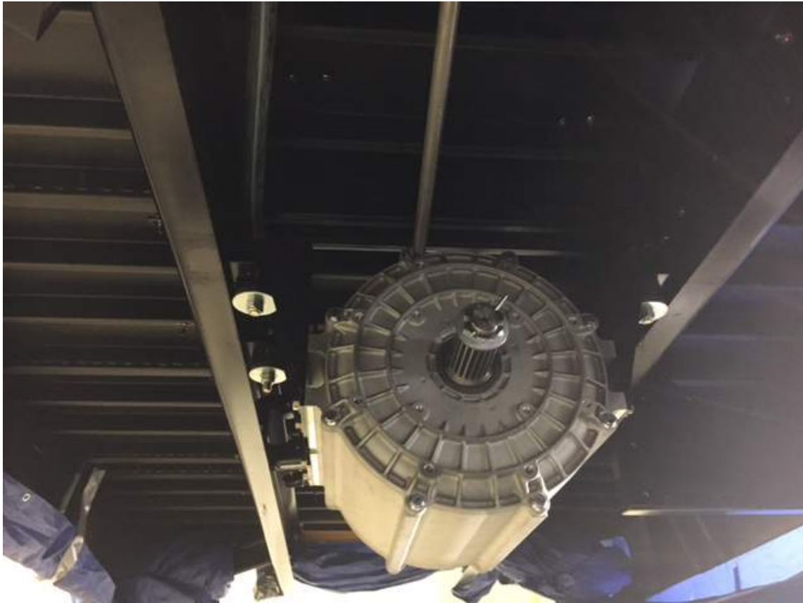
Figure II.5.1 - 3000NM Electric Motor Installed in Bus P1
