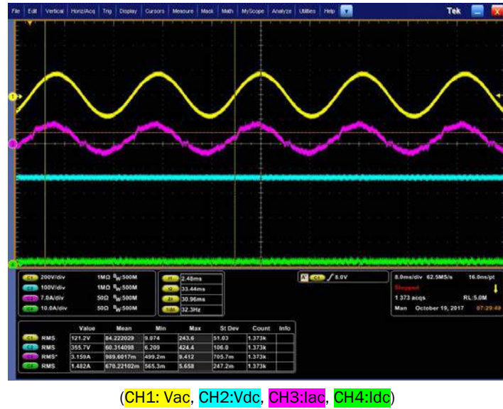
Figure II.1.3 - Level 1 charge waveform, Vout=350Vdc (CH1: Vac, CH2:Vdc, CH3:Iac, CH4:Idc)
