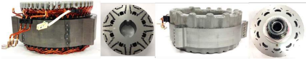
Figure I.7.7 - 2017 Prius motor stator, motor rotor, generator stator, and generator rotor.
