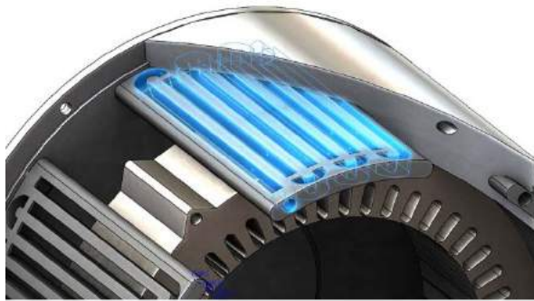
Figure I.15.6 - Cross section view of ORNL stator cooling jacket for computational fluid dynamics thermal and fluid analysis at NREL (left), transverse rupture test results comparing new and prior generation Ames magnets (right).
