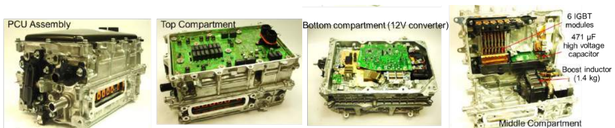
Figure I.7.1 - 2017 Prius PCU assembly and compartments.
