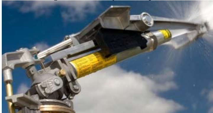
Figure 4-9: Gun Sprinkler System
