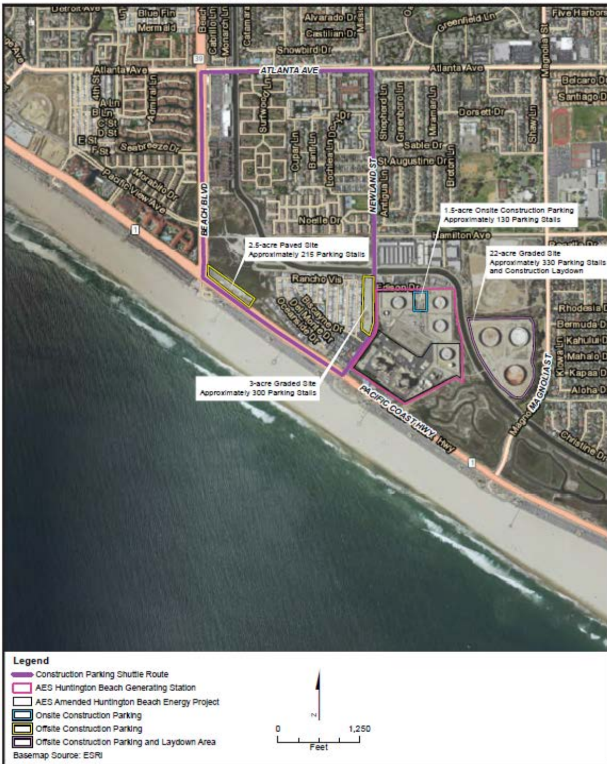
PROJECT DESCRIPTION - FIGURE 1 Amended Huntington Beach Energy Project - Construction / Laydown Parking Areas
