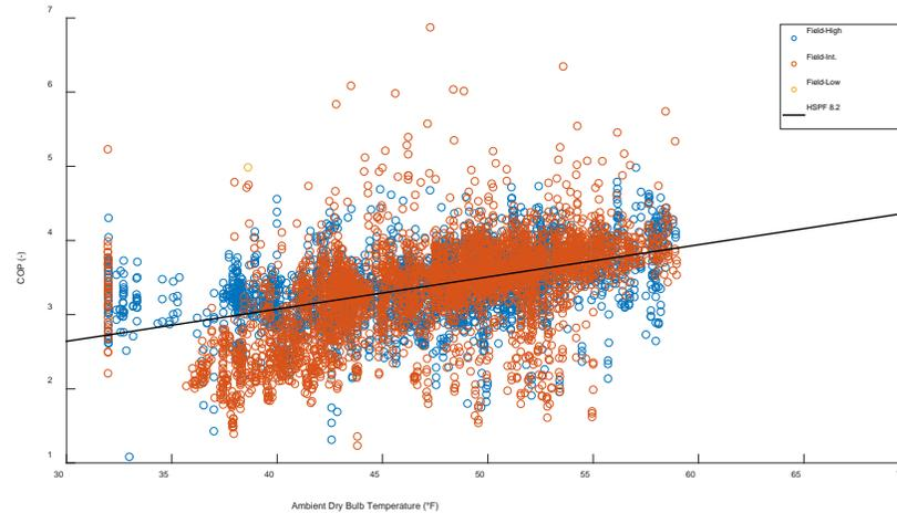
Unit cooling efficiency results @ PG&E site
