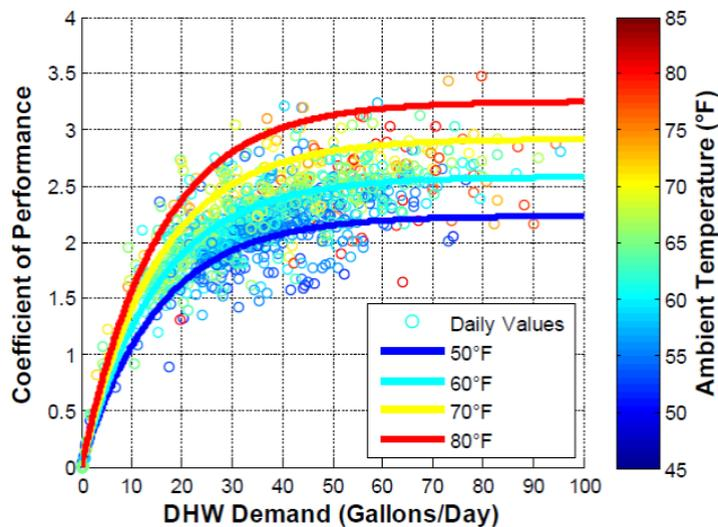
7. Figure 5. Efficiency of a 50-gal HPWH operating in heat pump mode
