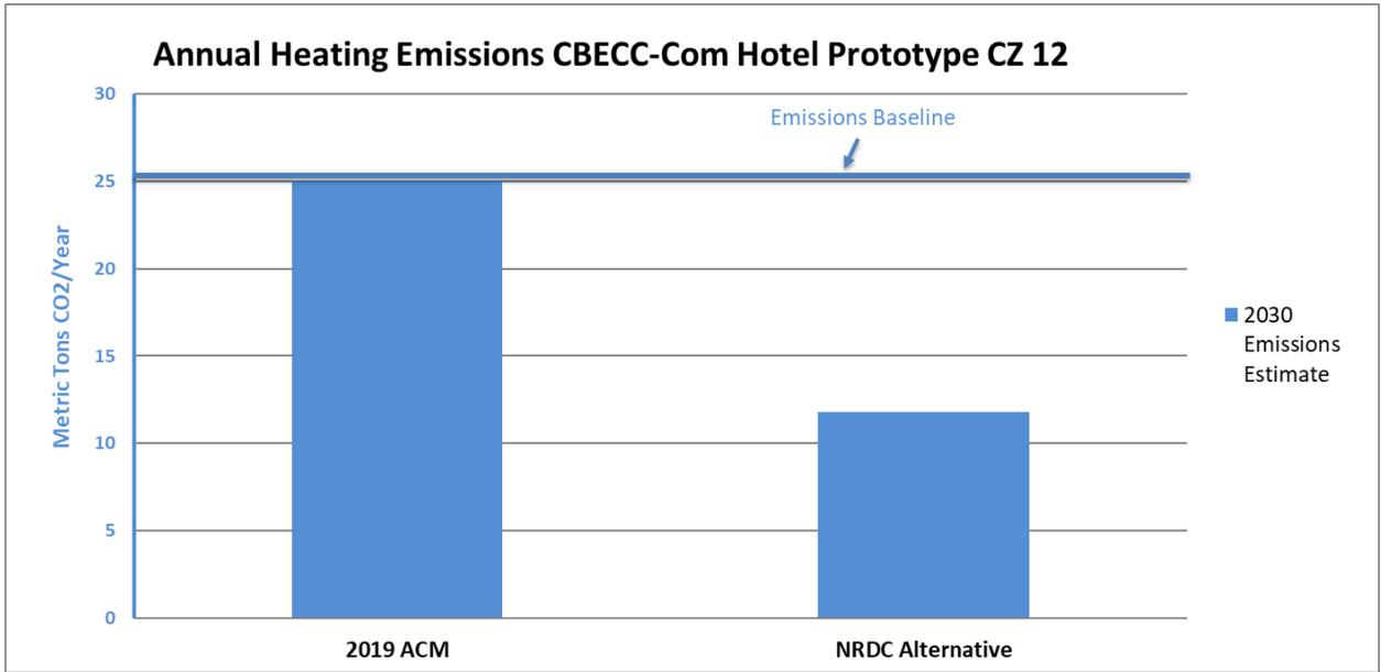
**Figure 5:** Space heating emissions for 2019 ACM baseline system and proposed baseline system type in small hotel prototype in Climate Zone 12.
