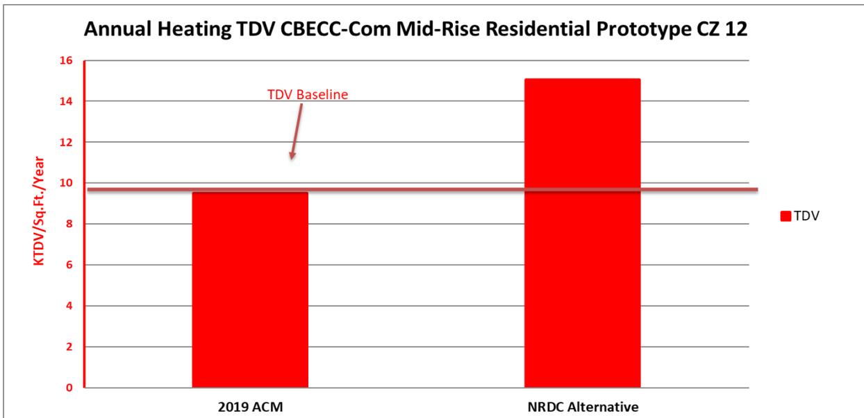
**Figure 2:** TDV Energy for 2019 ACM baseline system and proposed baseline system type in a 4-story mid-rise residential prototype in Climate Zone 12.
