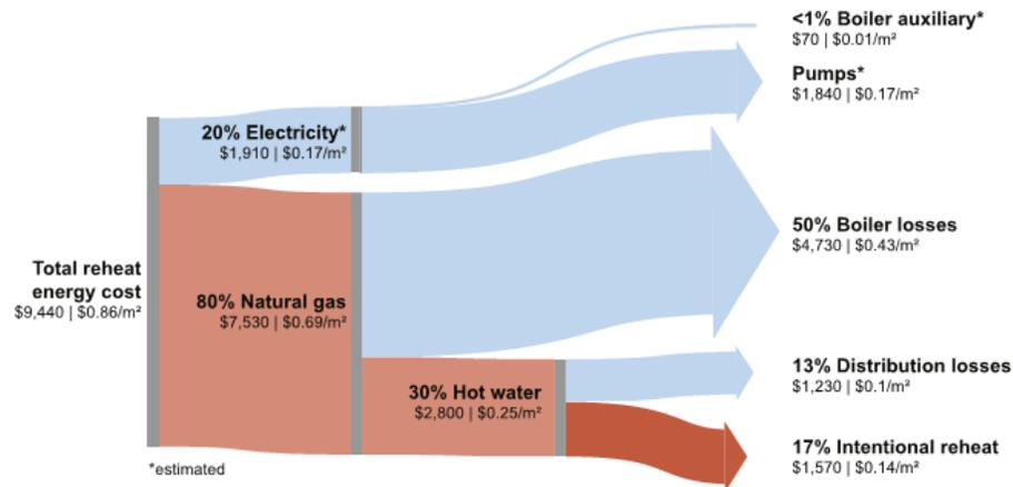
**Figure 9:** Total heating energy use compared to intentional reheat energy in a 120,000 sq. ft. Bay Area office building during operational hours.<sup>8</sup>
