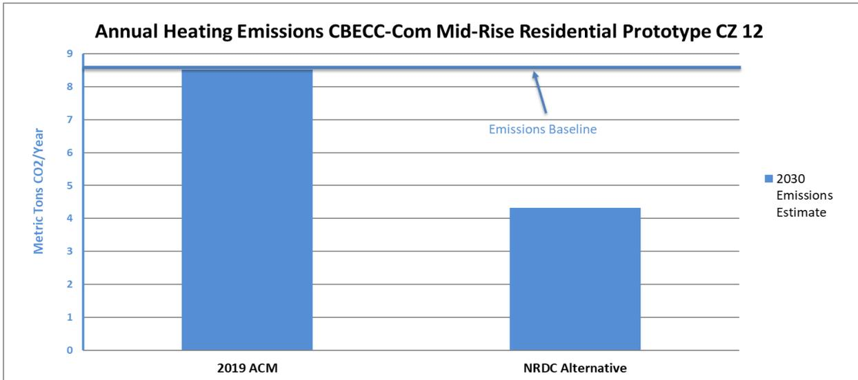
**Figure 1:** Space heating emissions for 2019 ACM baseline system and proposed baseline system type in a 4-story mid-rise residential prototype in Climate Zone 12.
