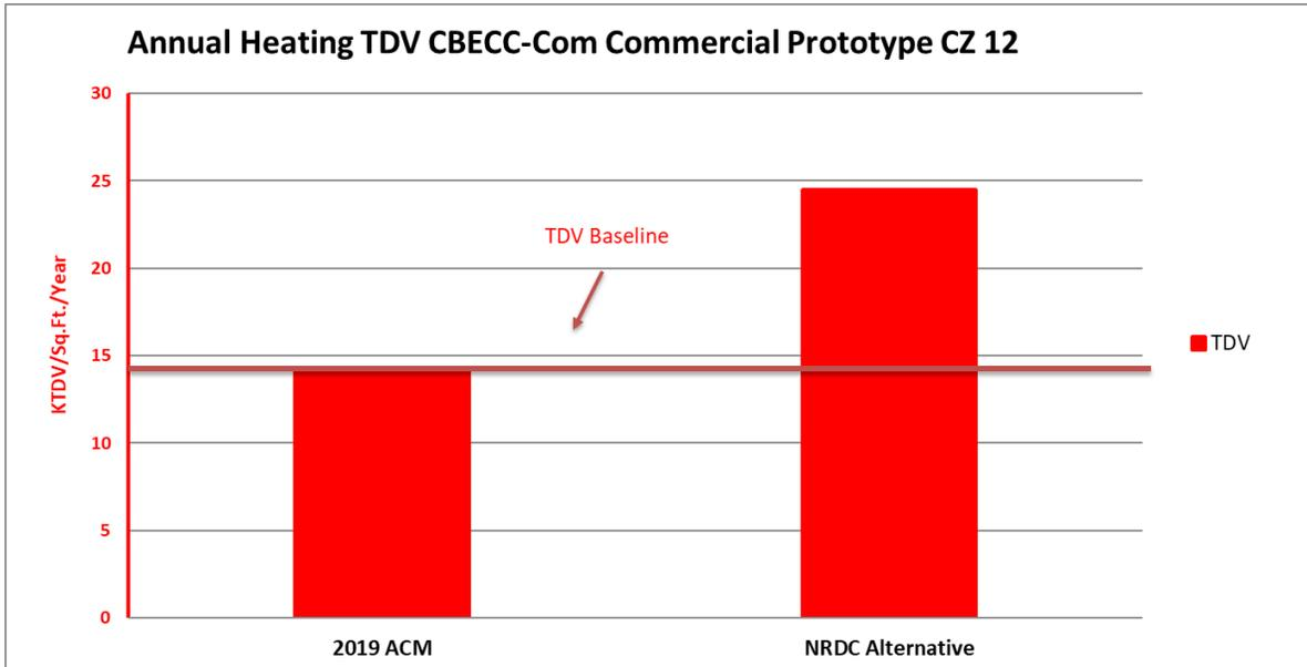
**Figure 8:** TDV Energy for 2019 ACM baseline system and proposed baseline system type in the medium office prototype in Climate Zone 12.
