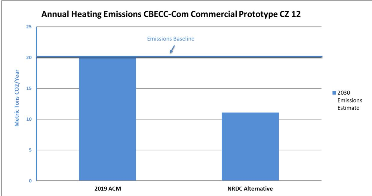
**Figure 7:** Space heating emissions for 2019 ACM baseline system and proposed baseline system type in the medium office prototype in Climate Zone 12.
