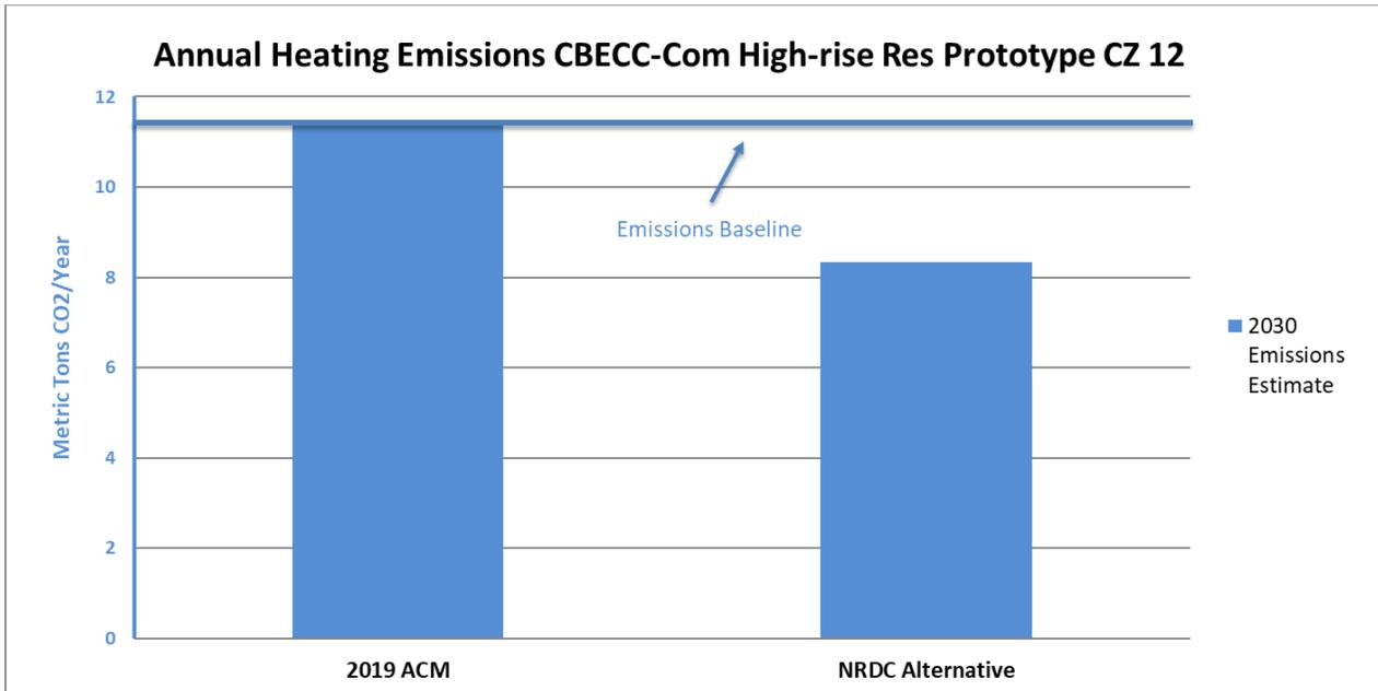
**Figure 3:** Space heating emissions for 2019 ACM baseline system and proposed baseline system type in a 9-story high-rise residential prototype in Climate Zone 12.
