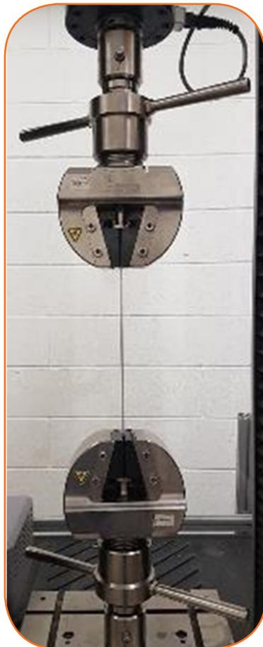
Figure 23: Typical Strand Tensile Testing Setup
