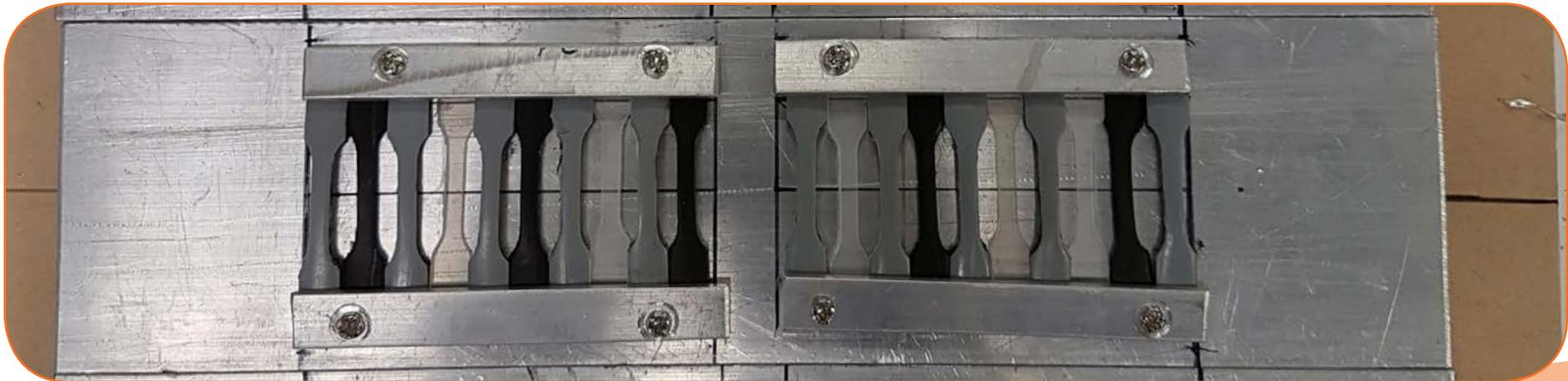
Figure 17: UV Testing Specimen Plate
