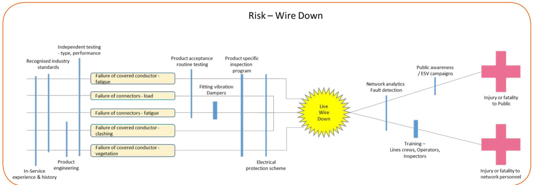
Figure 58: Wire Down- Threat Barrier Diagram
