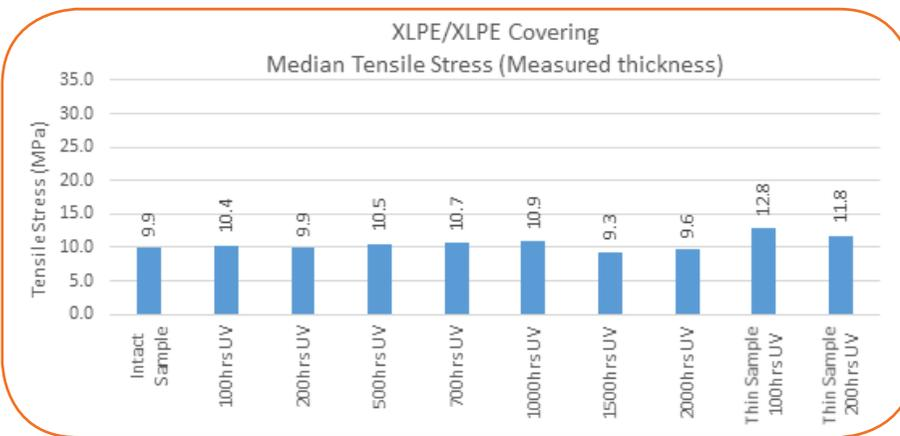
Figure 47: XLPE/XLPE Covering Median Tensile Stress (Measured thickness)
