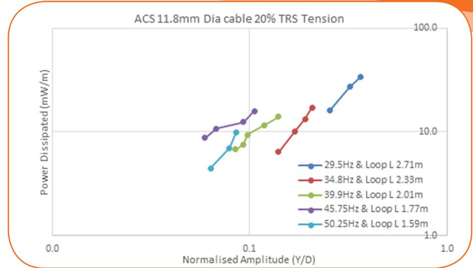
Figure 29: 7/2.12 ACS Vibration Testing Result at 20% UTS Tension
