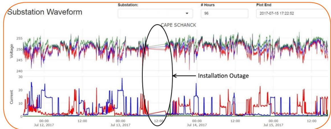
Figure 60: Voltage and Current Profile Pre and Post Covered Conductor Installation
