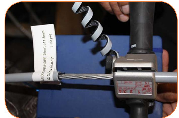
Figure 25: Stripping Test Example
