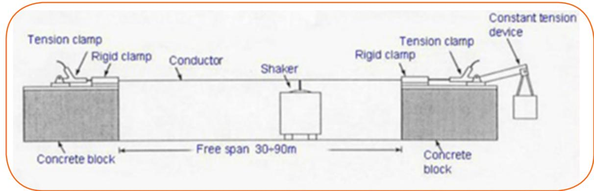
Figure 26: Test span for conductor self-damping measurement
