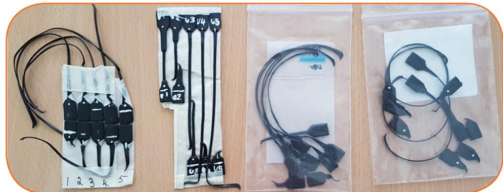
Figure 42: United Energy Cable sample- Photo order: Intact sample, 100hrs UV, 200hrs UV & 500hrs UV
