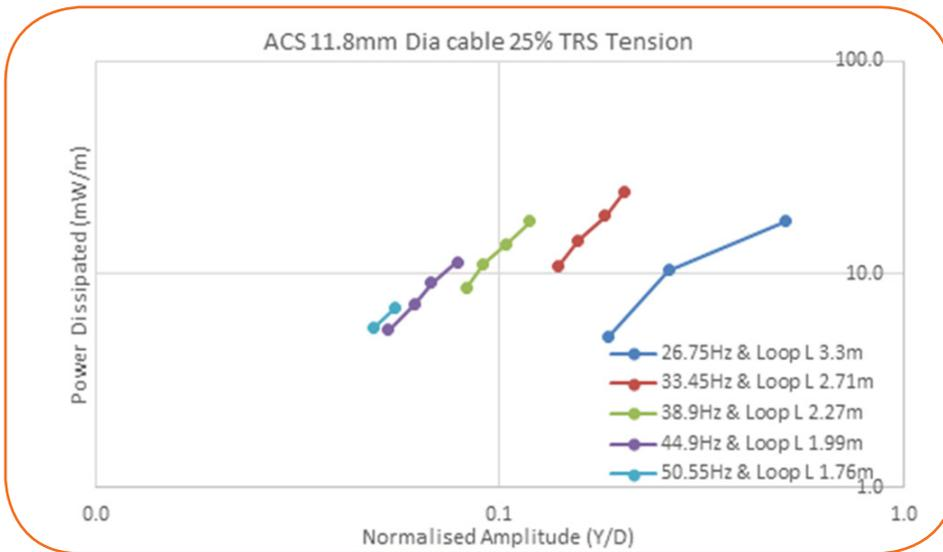
Figure 30: 7/2.12 ACS Vibration Testing Result at 25% UTS Tension
