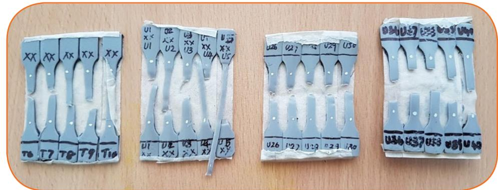
Figure 41: XLPE/XLPE Covered Conductor sample- Photo order: Intact sample, 100hrs UV, 200hrs UV & 500hrs UV
