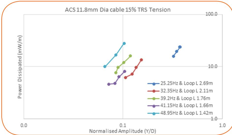
Figure 28: 7/2.12 ACS Vibration Testing Result at 15% UTS Tension
