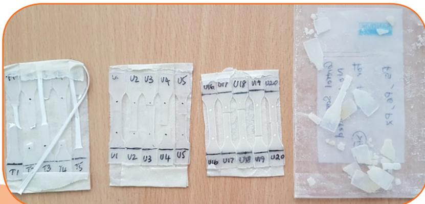
Figure 43: Non-UV treated ABS Material\* - Photo order: Intact sample, 100hrs UV, 200hrs UV & 500hr
