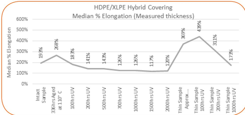
Figure 48: HDPE/XLPE Hybrid Covering Median % Elongation (Measured thickness)
