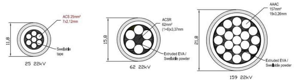
Figure 11: Amokabel Covered Conductor Cross-Section Diagrams
