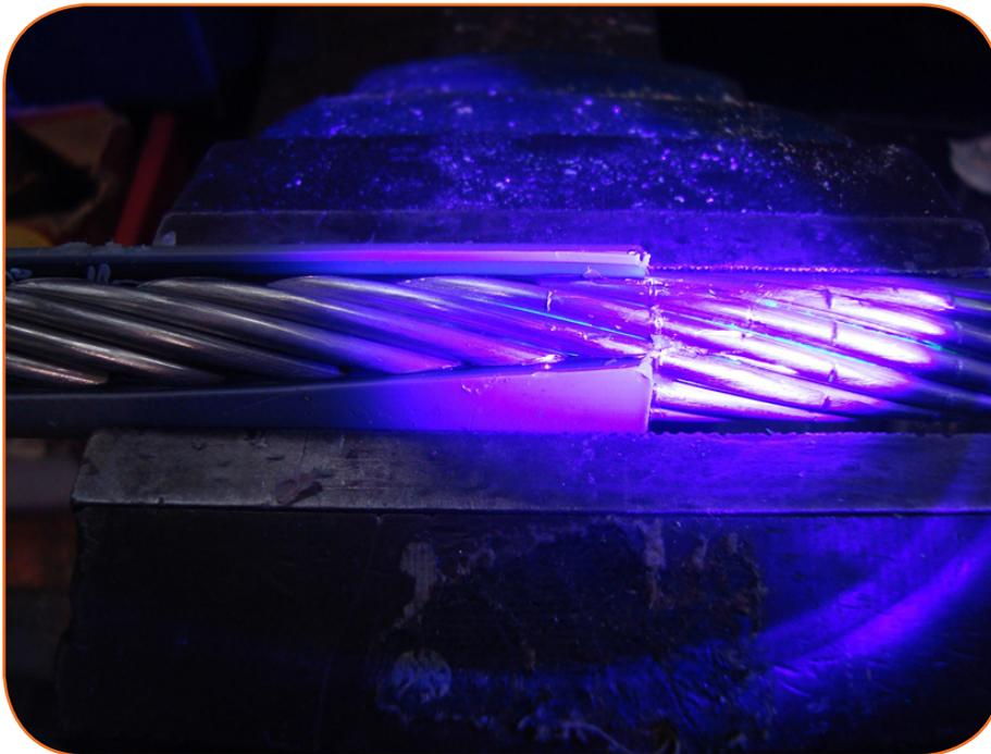
Figure 19: Typical View During Water Blocking Testing
