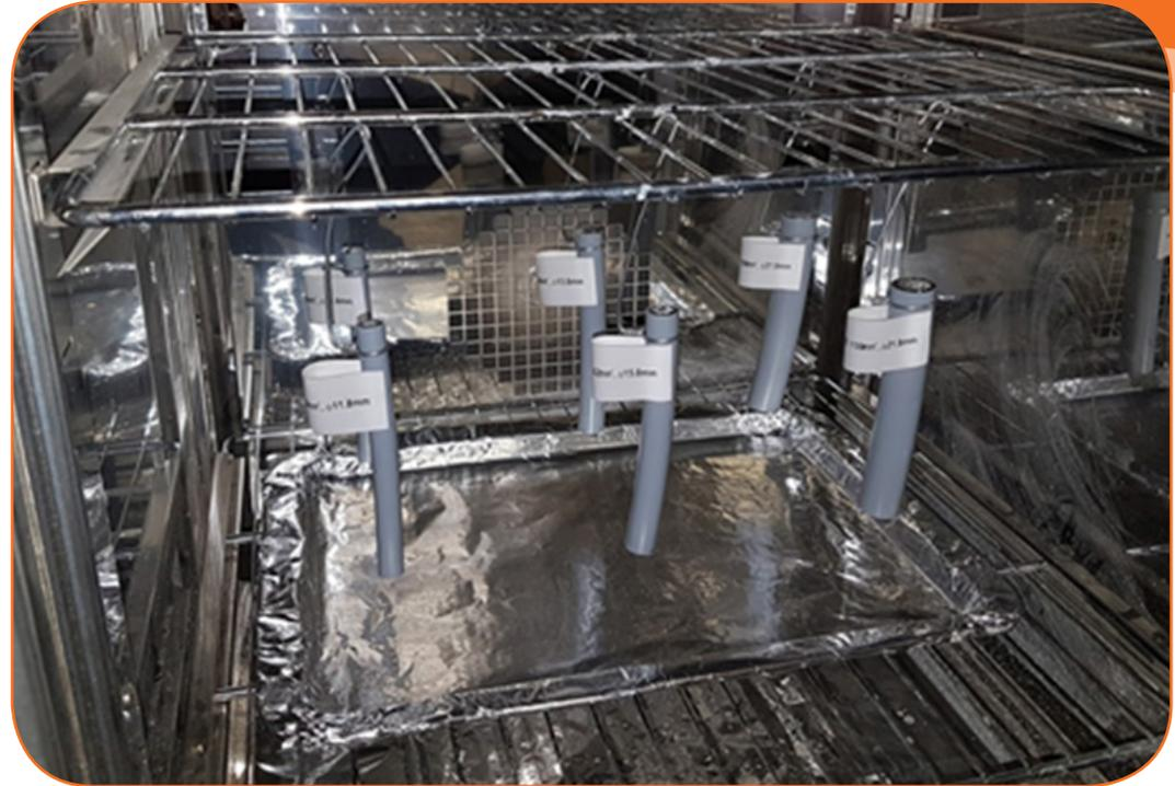
Figure 22: Dripping Test Setup
