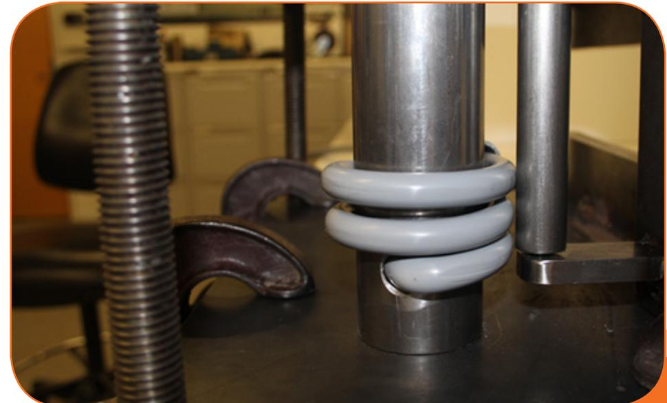
Figure 34: Bending Test at Low Temperature Example
