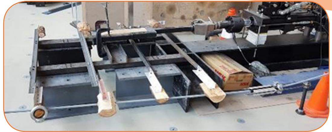
Figure 35: Abrasion Testing Rig
