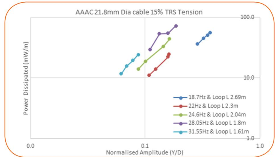
Figure 31: 19/3.37 AAC Vibration Testing Result at 15% UTS Tension
