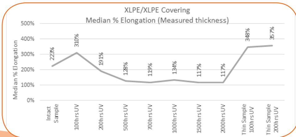
Figure 49: XLPE/XLPE Covering Median % Elongation (Measured thickness)
