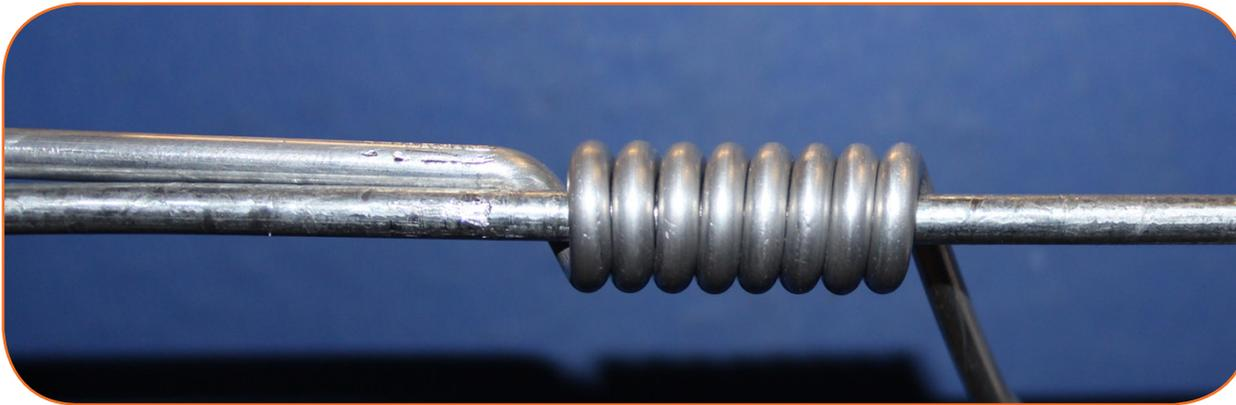
Figure 24: Strand Wrapping Test Example
