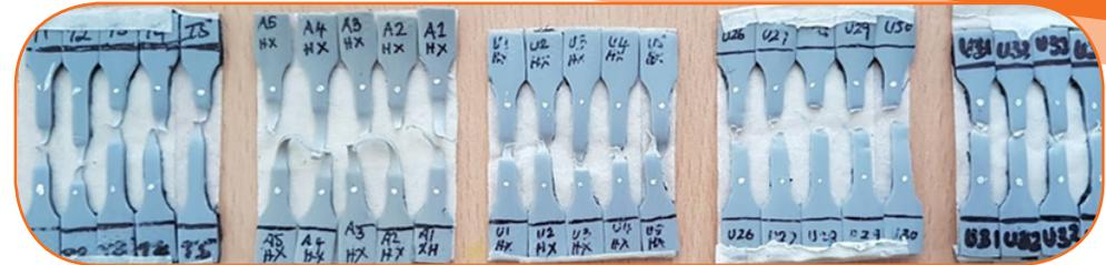
Figure 40: HDPE/XLPE Covered Conductor sample- Photo order: Intact sample, 336hrs aging test, 100hrs UV, 200hrs UV & 500hrs UV
