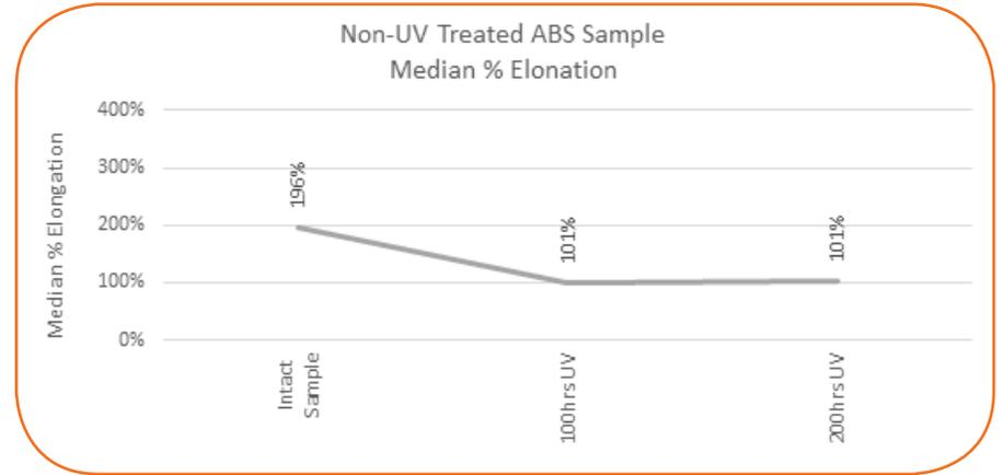
Figure 52: Non-UV Treated ABS Sample Median % Elongation
