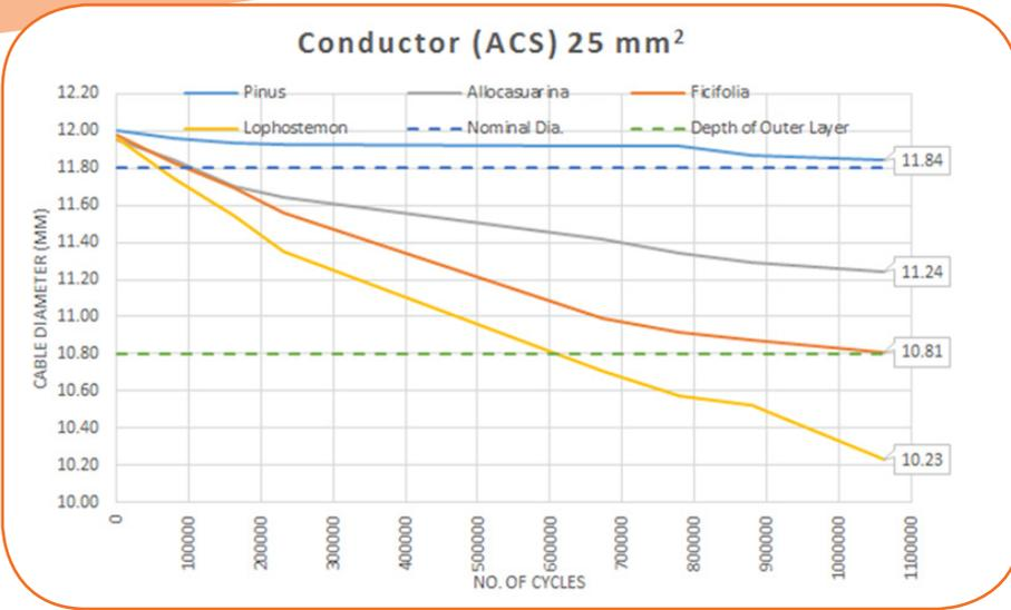
Figure 37: 7/2.12 ACS Abrasion Testing Results
