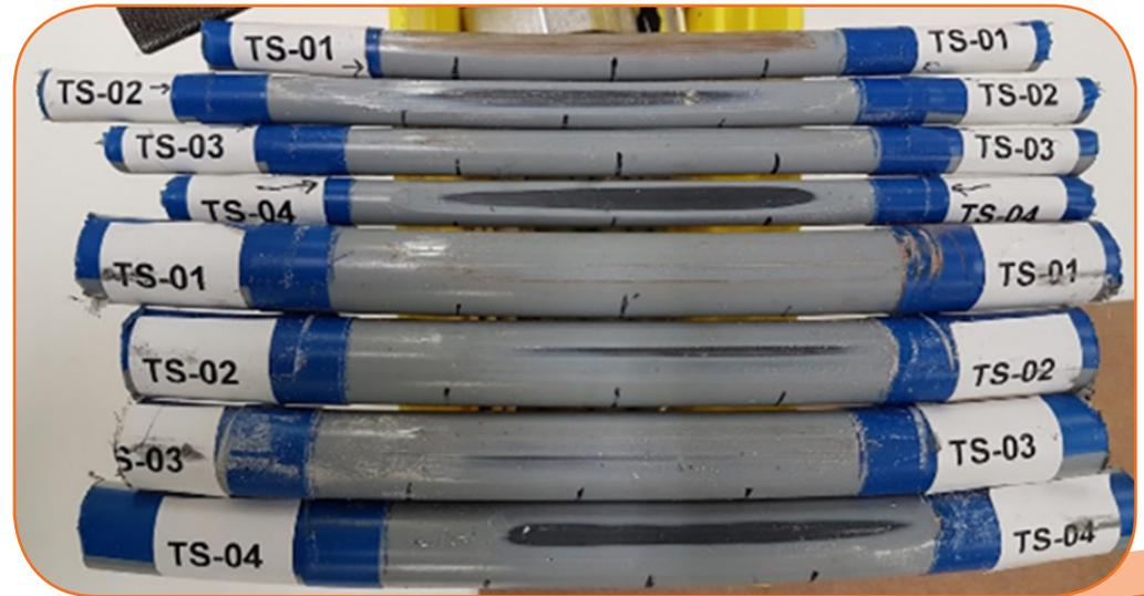
Figure 39: Abrasion Test Specimens Post Test
