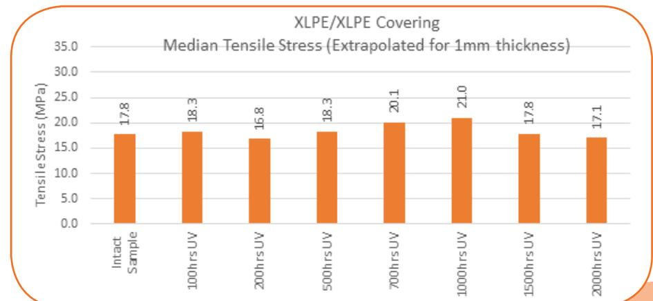
Figure 46: XLPE/XLPE Covering Median Tensile Stress (Extrapolated for 1mm thickness)
