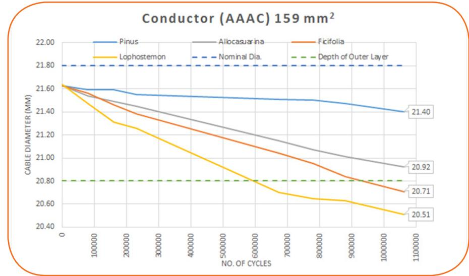
Figure 38: 19/3.37 AAAC Abrasion Testing Result
