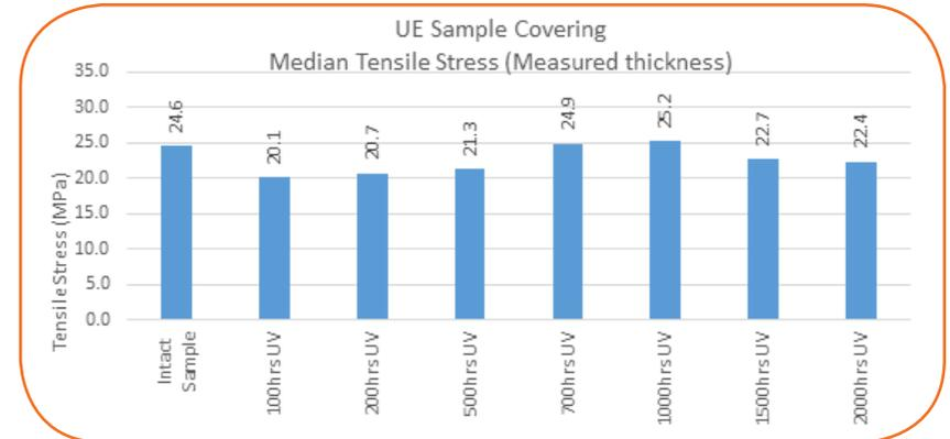
Figure 50: UE Sample Covering Median Tensile Stress (Measured thickness)
