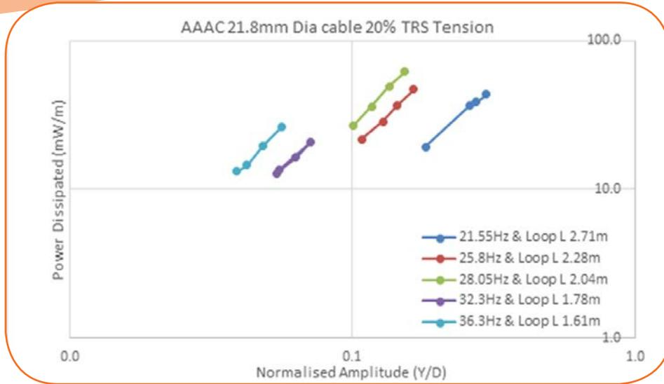
Figure 32: 19/3.37 AAAC Vibration Testing Result at 20% UTS Tension
