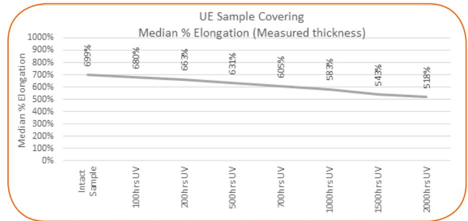
Figure 51: UE Sample Covering Median % Elongation (Measured thickness)
