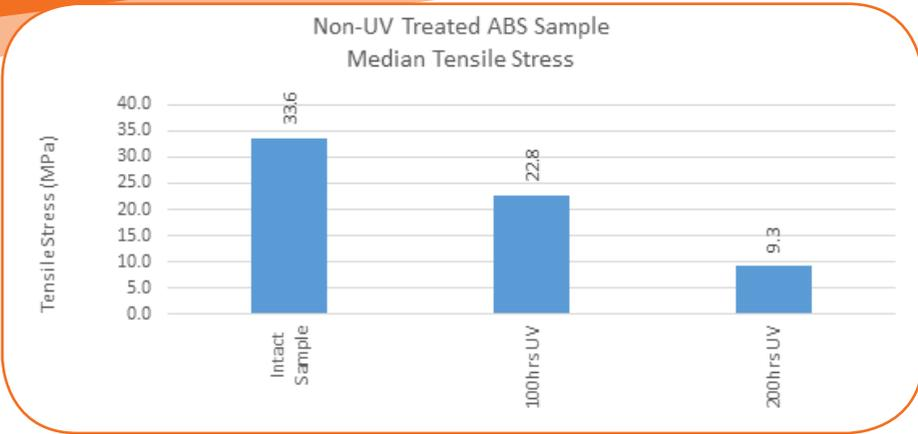
Figure 53: Non-UV Treated ABS Sample Median Tensile Stress
