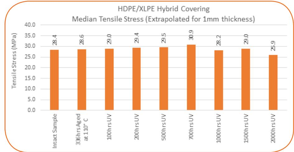
Figure 44: HDPE/XLPE Hybrid Covering Median Tensile Stress (Extrapolated for 1mm thickness)
