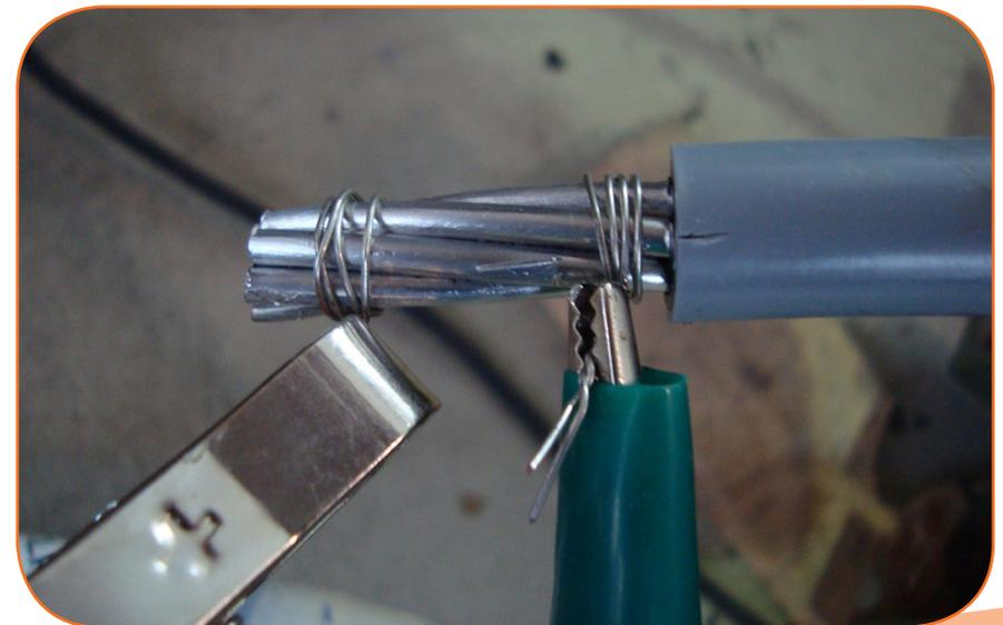
Figure 18: Interstrand Conductivity Test Setup
