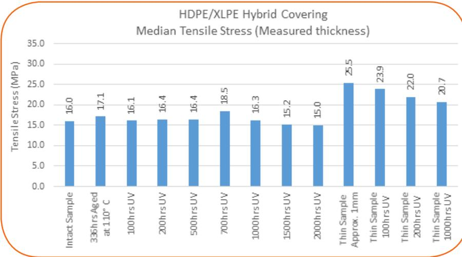
Figure 45: HDPE/XLPE Hybrid Covering Median Tensile Stress (Measured thickness)
