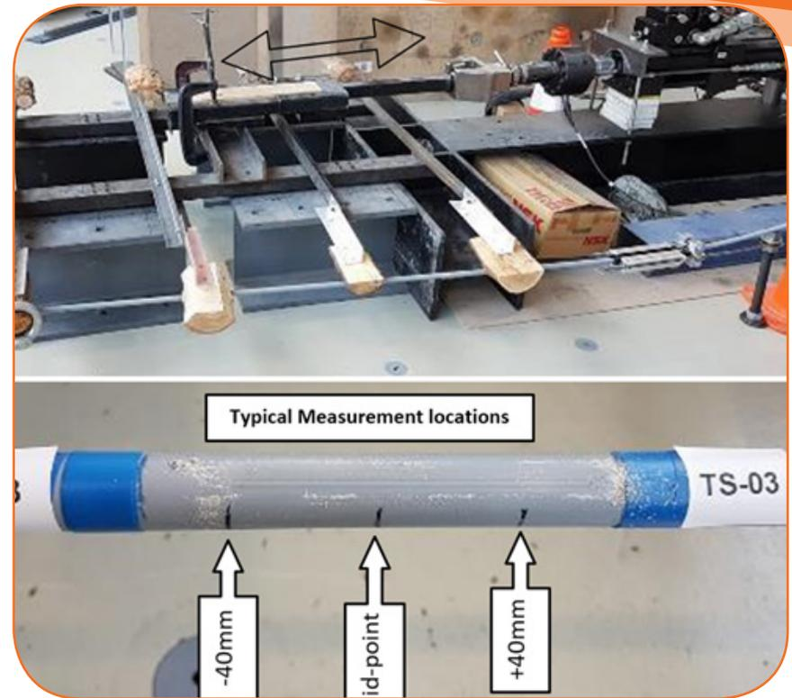
Figure 14: Abrasion test setup showing typical test specimen with locations of measurement of diameters during testing
