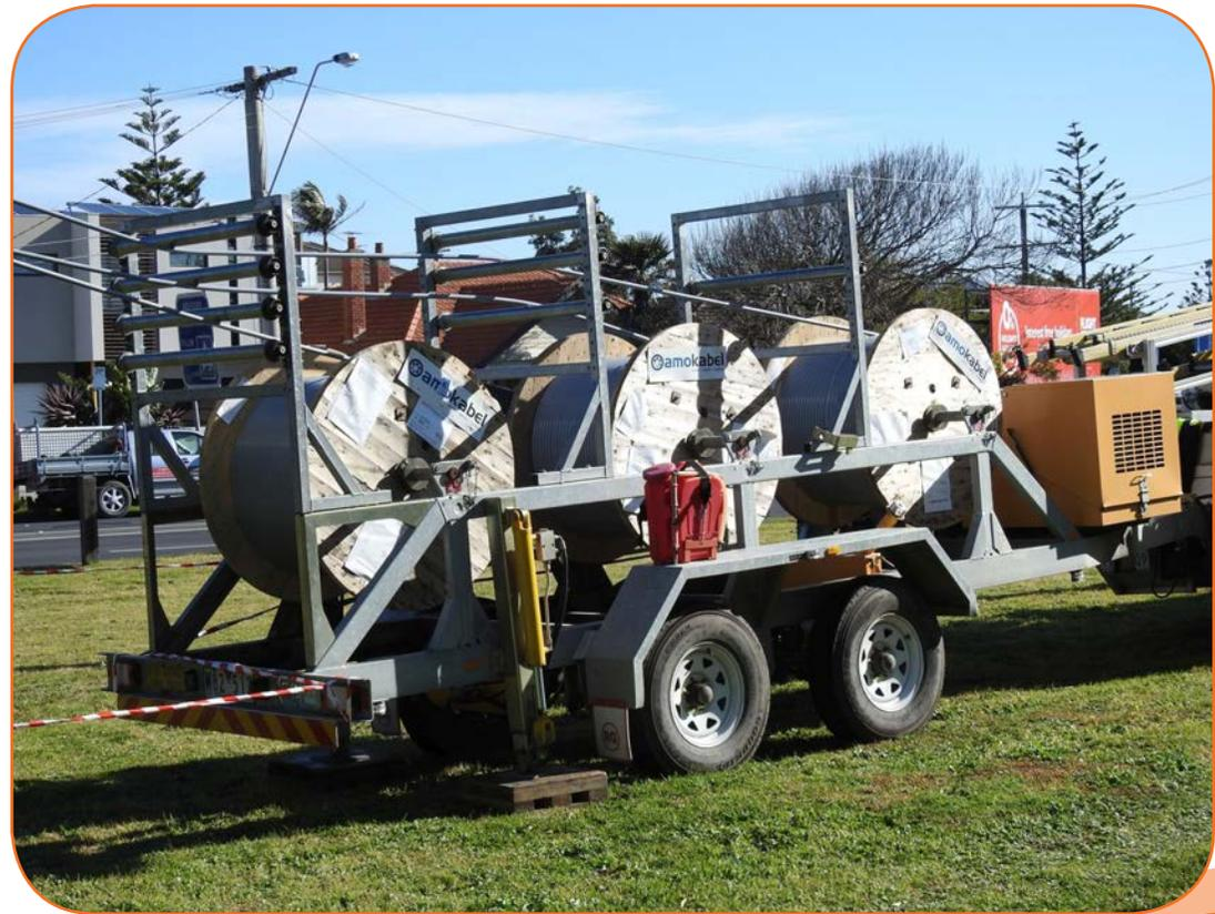
Figure 4: Amokabel covered conductor drums on stringing trailer
