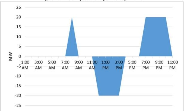
Figure 17 below shows the charge and discharge profile used to model a generic Li-Ion BESS
