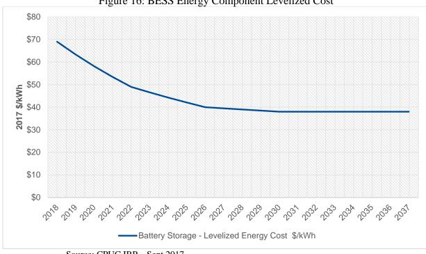
Figure 16: BESS Energy Component Levelized Cost
