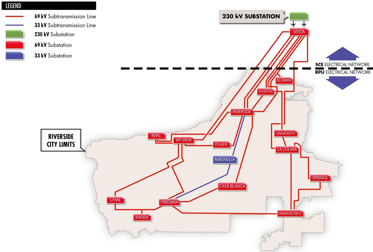
Figure 4.2.1. Existing RPU sub transmission electrical system.
