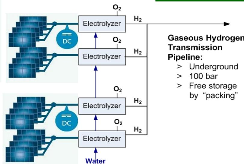
Solar plants may be dedicated to Hydrogen fuel production, with no connection to the electricity grid, without costly conversion systems and infrastructure to deliver grid-quality AC or DC.
