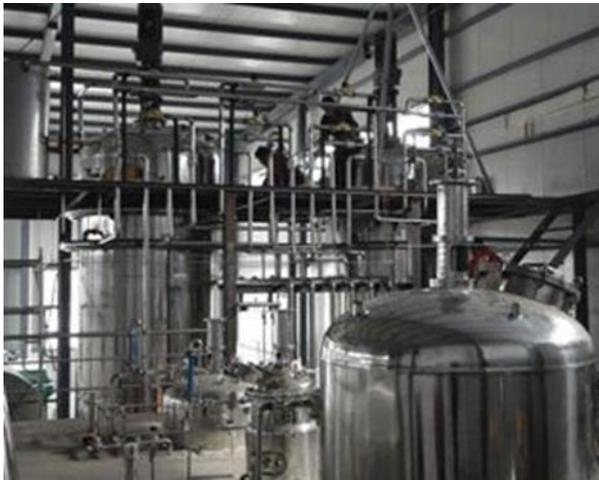
Syngas is cleaned, cooled, and sent to a bioreactor that converts it to a crude ethanol/water mixture;
