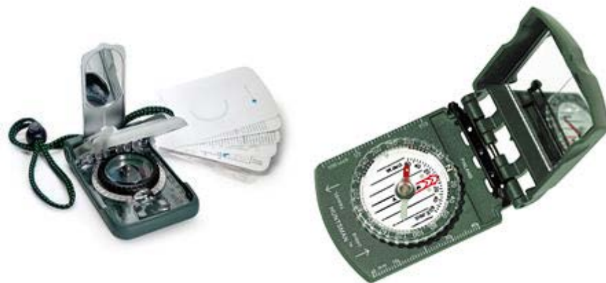
Figure C.4: Compass With a Sighting Feature
