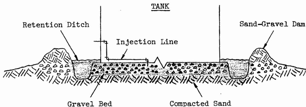
\* Shaded portion indicates area saturated with seal oil.
