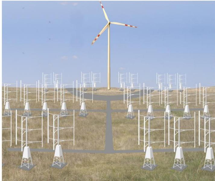
Figure 2 – Here is how three rows of Harvester VAWTs would look like with a distance of 70+ meters between each row and with the last row being directly under the HAWT rotor.
