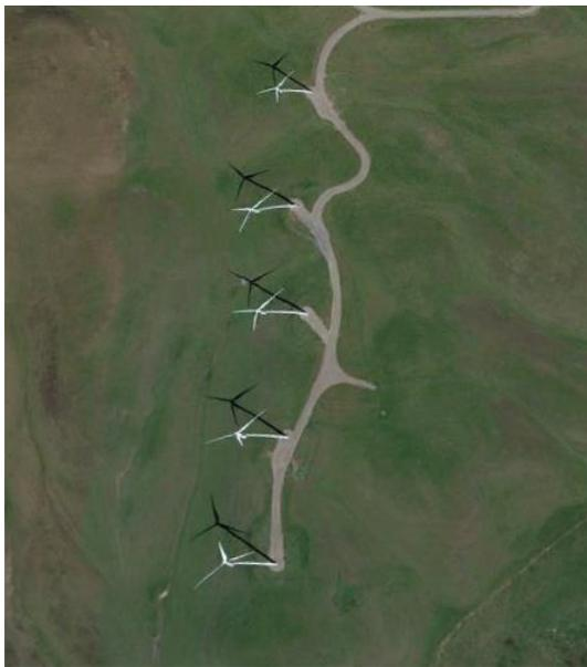
Figure 1 - The distance between HAWTs in this typical row in the Solano Wind Resource Area is 185m and the average distance to the downwind row being 750m.
