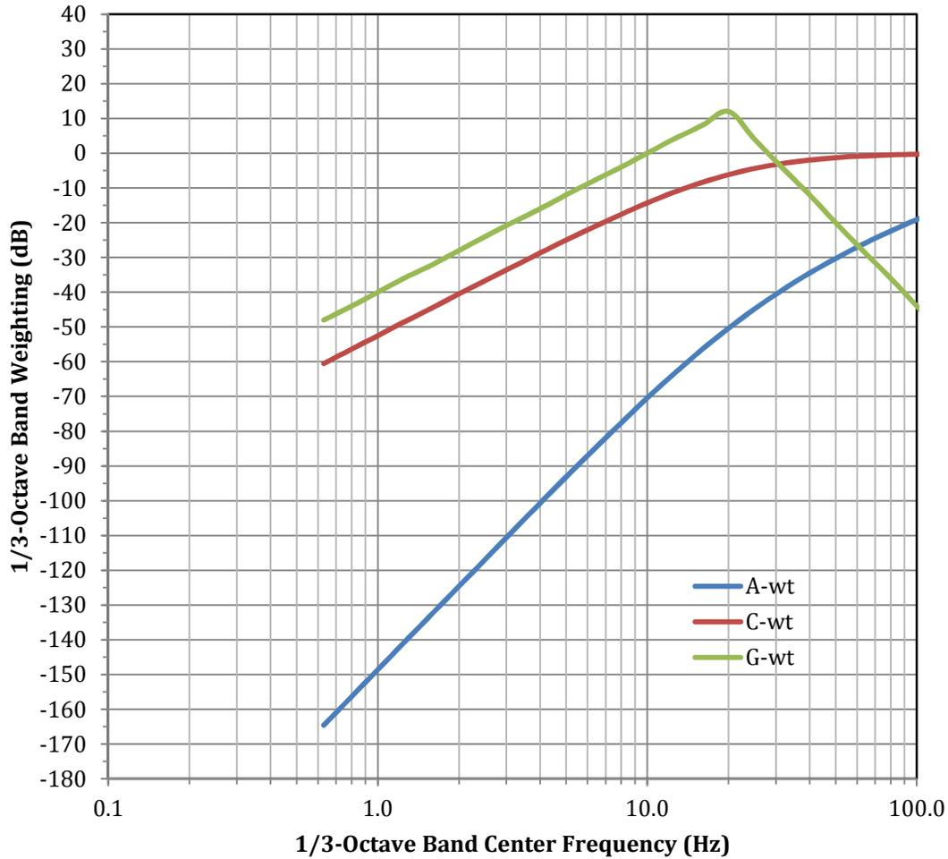
Figure 6 A, C and G Spectral Weighting Curves
