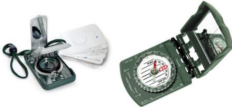
Figure C.4: Compass With a Sighting Feature
