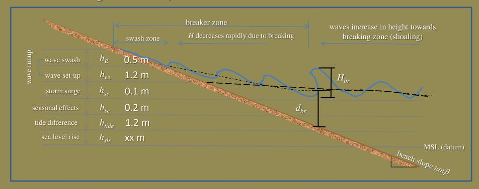
flood level is the combination of rSLR + tides + seasonal effects + storm surge + wave setup + wave runup + fluvial discharge backflow (not shown)
