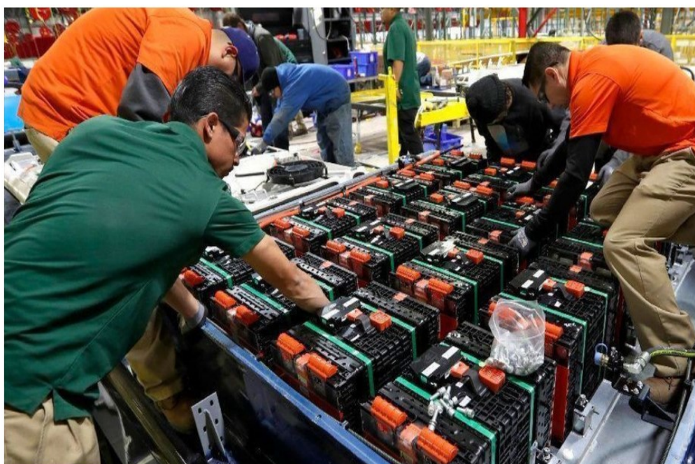
Workers install batteries on top of a bus destined for UC Irvine. BYD's business began with production of cellphone batteries. (Mel Melcon / Los Angeles Times)
