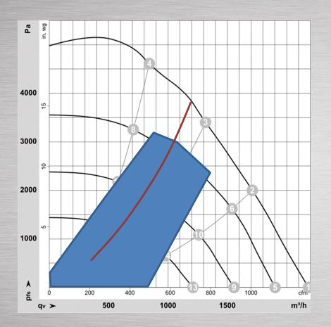
The peak efficiency for fans often stops before the maximum RPM is reached. Many combustion systems use the full range of RPMs to maximize modulation (turndown ratio).
