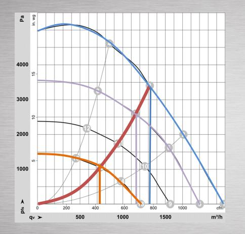
The point where the fan curve intersects the resistance curve for the combustion appliance determines the air flow rate.
