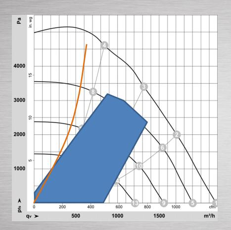
**High efficiency heat** exchangers create turbulence and enhance surface contact to maximize heat transfer. This creates high pressure drops and may go outside the peak fan efficiency curve.
