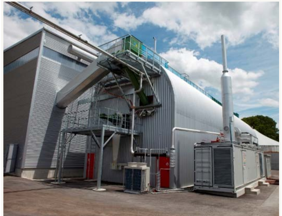
HZIU Kompogas high-solids anaerobic digestion system designed to meet SLO County organics diversion goals
