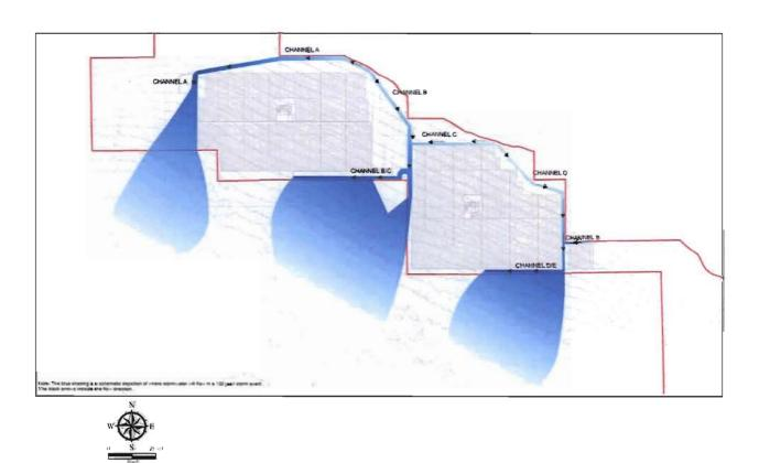
1. Drainage Plan for Genesis Solar Energy Project, showing dispersal points and pattern of shallow, dispersed overland flow. (RSA, Soil and Water Figure 19.)
