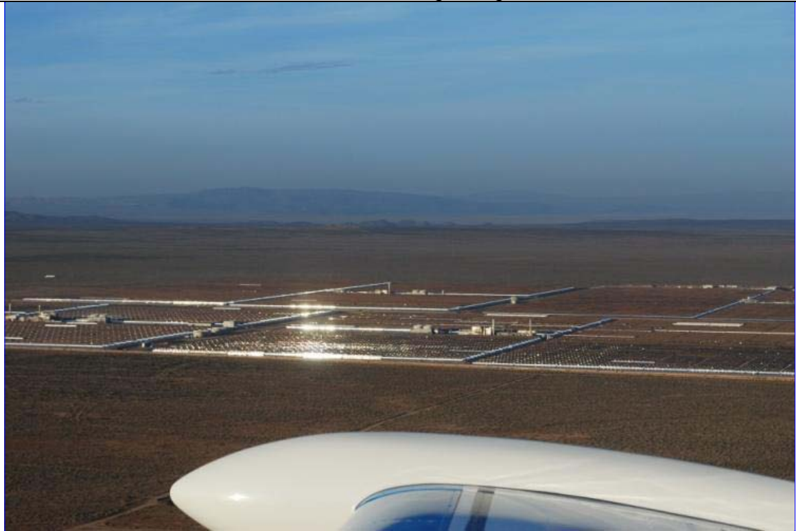
Figure 6. Typical View of the Glint/Glare from an Operating Solar Array with a Low Sun Angle on Close Approach
