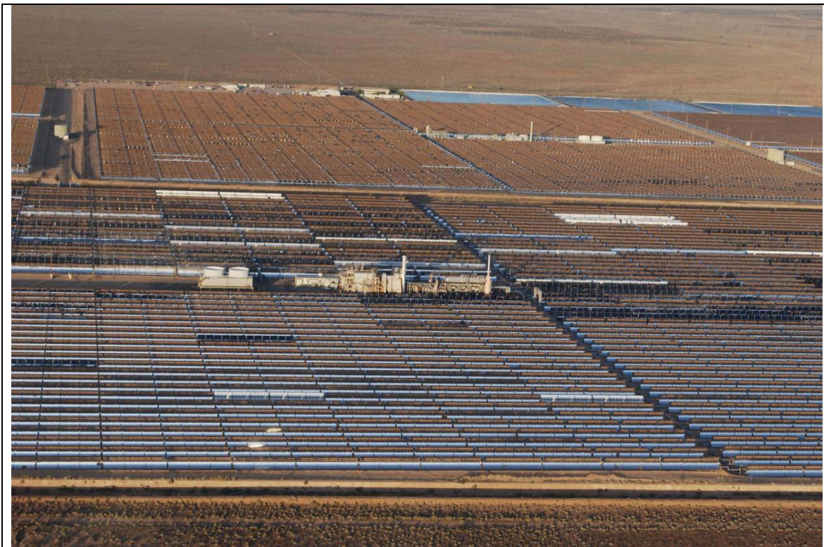
Figure 8. Typical View of Localized Glint/Glare from an Operating Solar Array with a Low Sun Angle. See the local bright spots on Rows 3 and 5 in the left foreground. The larger apparent discontinuities in the solar array are from mirrors not aligned with the surrounding arrays.
