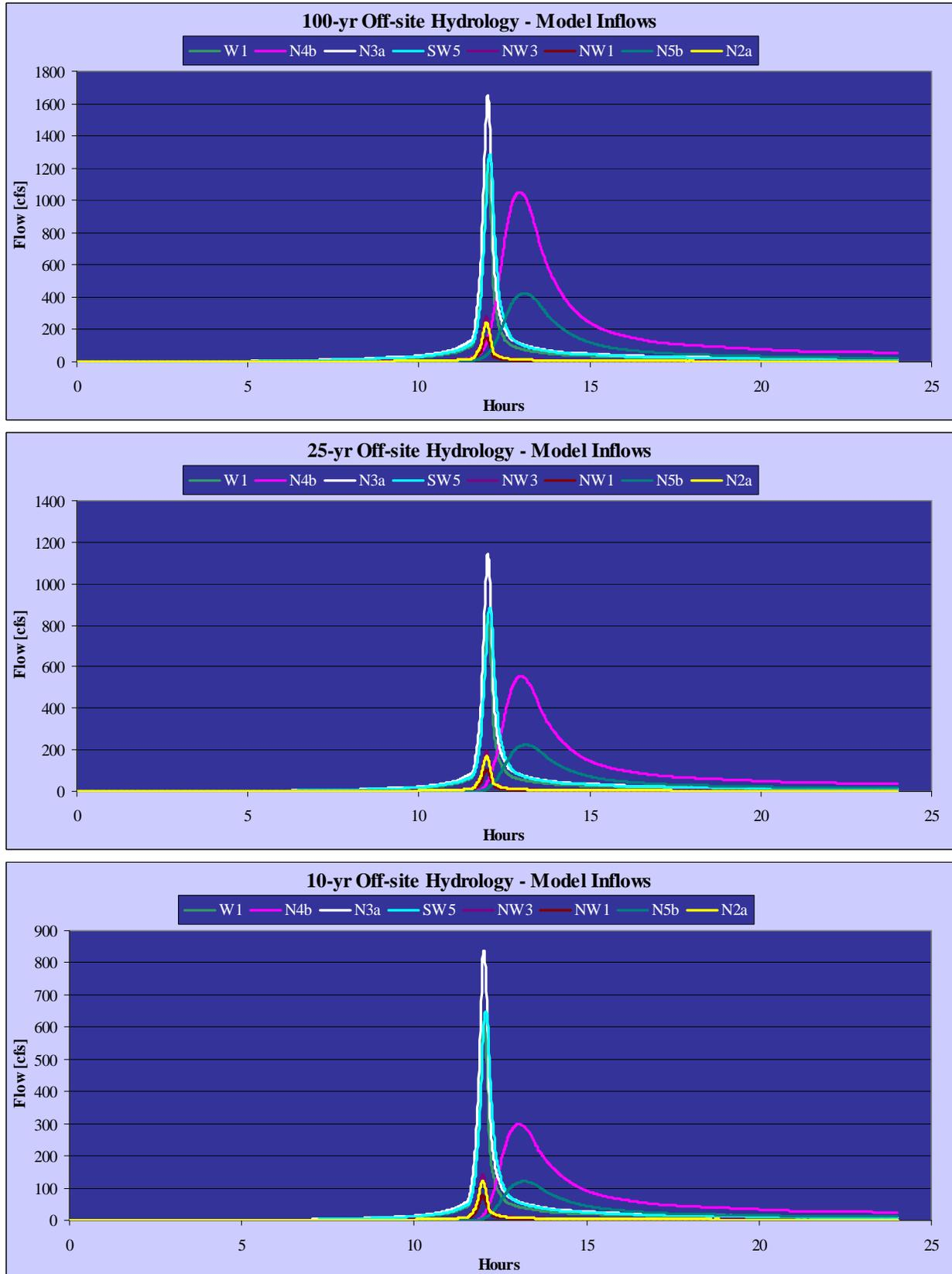
**Figure 3. Inflow hydrographs for 100, 25 and 10 year hydrologic events**
