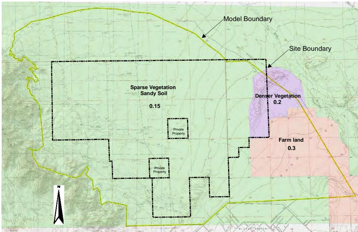
Figure 2. Spatial distribution of overland flow roughness coefficients
