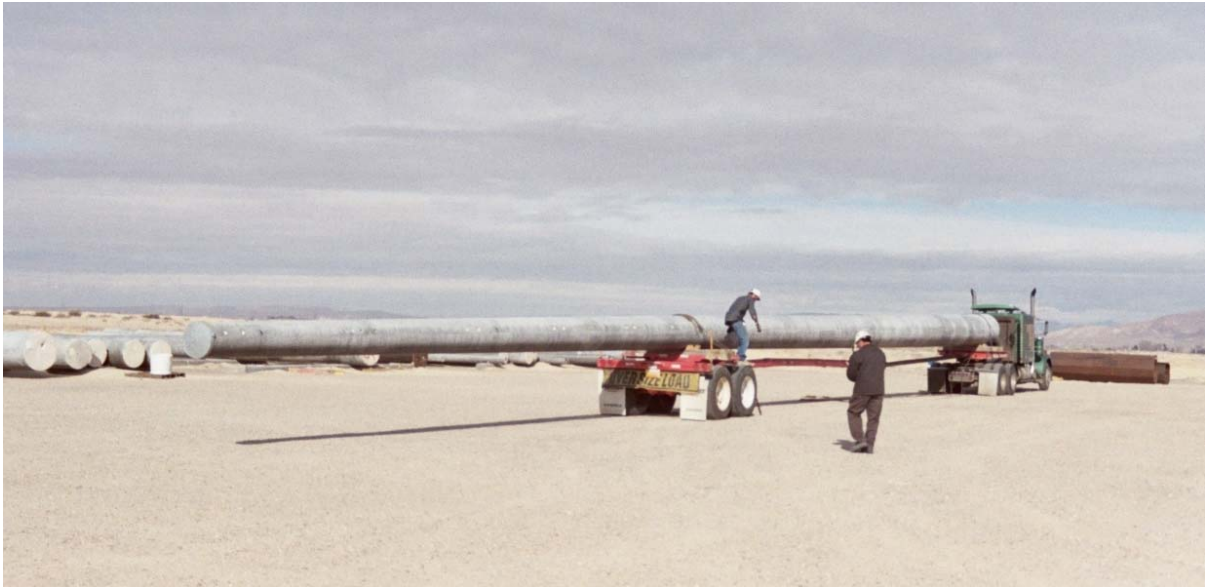
Figure 3. A 130-foot-long spun concrete pole being secured on a pole trailer for transport; note the approximately 45-foot overhang on the back
