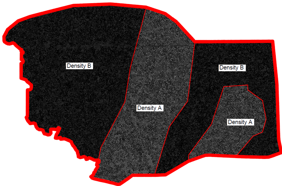
Figure 2 MIKE 21 mesh representing the project site with areas of higher density indicated.
