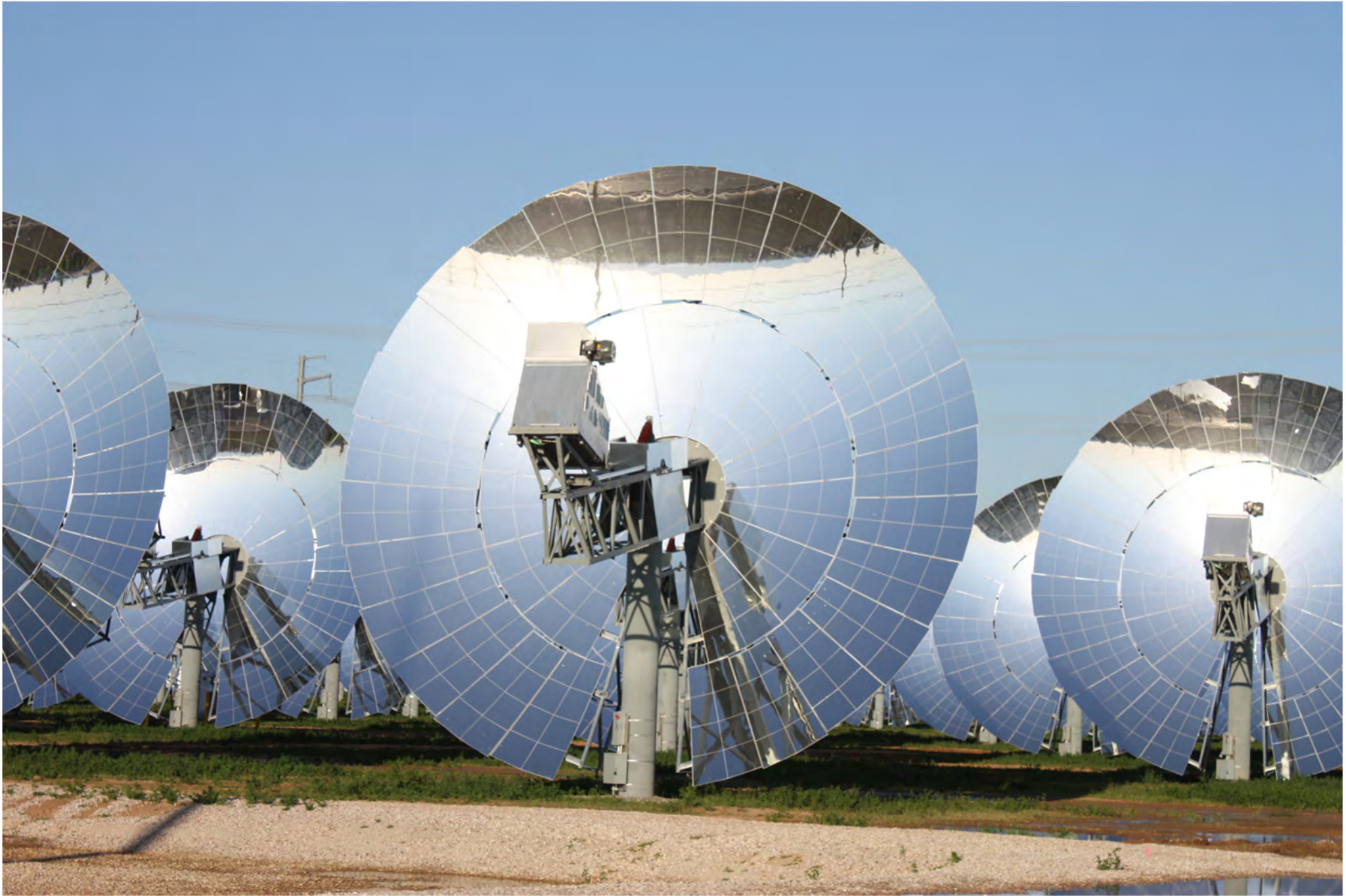
Imperial Valley Solar Project Examples of Glint Hidden by PCU Figure 6
