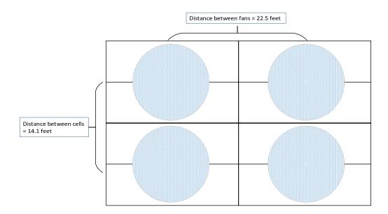
The model results presented here use the distance between the cells, 14.1 feet, and the number of cells, 8, to calculate the velocity of the merged plumes.
