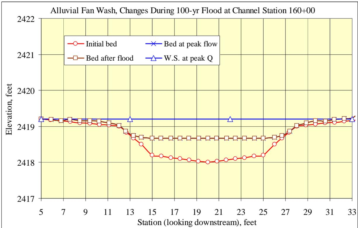
Figure 13. Simulated changes for sample channel cross sections
