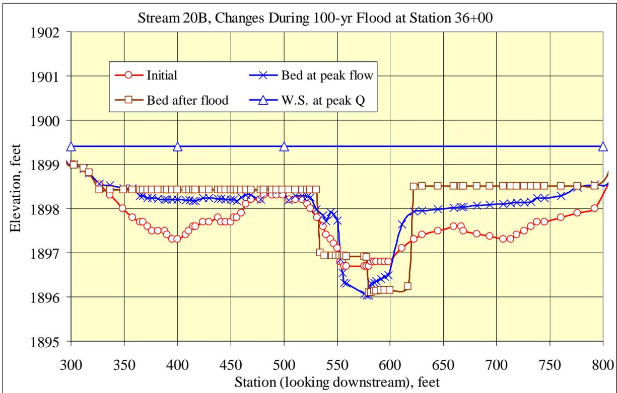
Figure 31(continued). Simulated cross sectional changes at sample cross sections along steam 20B
