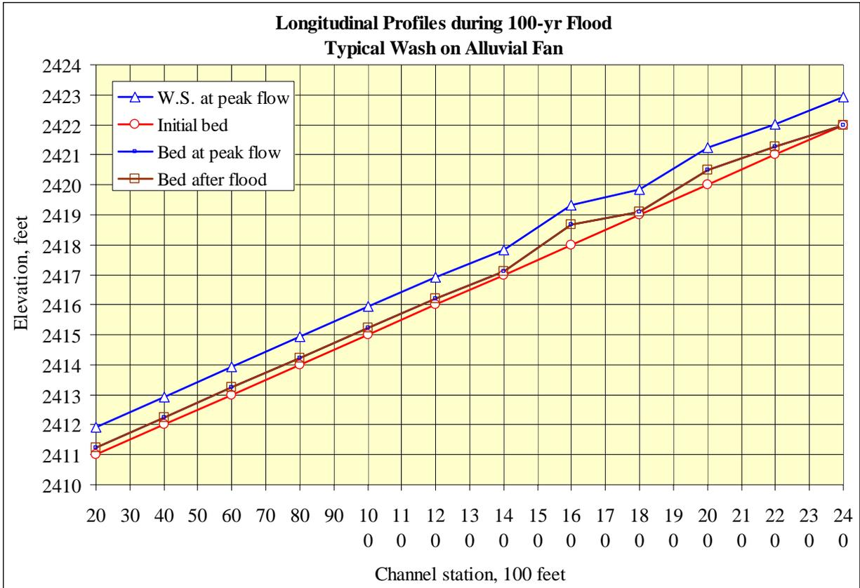
Figure 11. Water-surface and channel bed profile changes during 100-yr flood for sample wash
