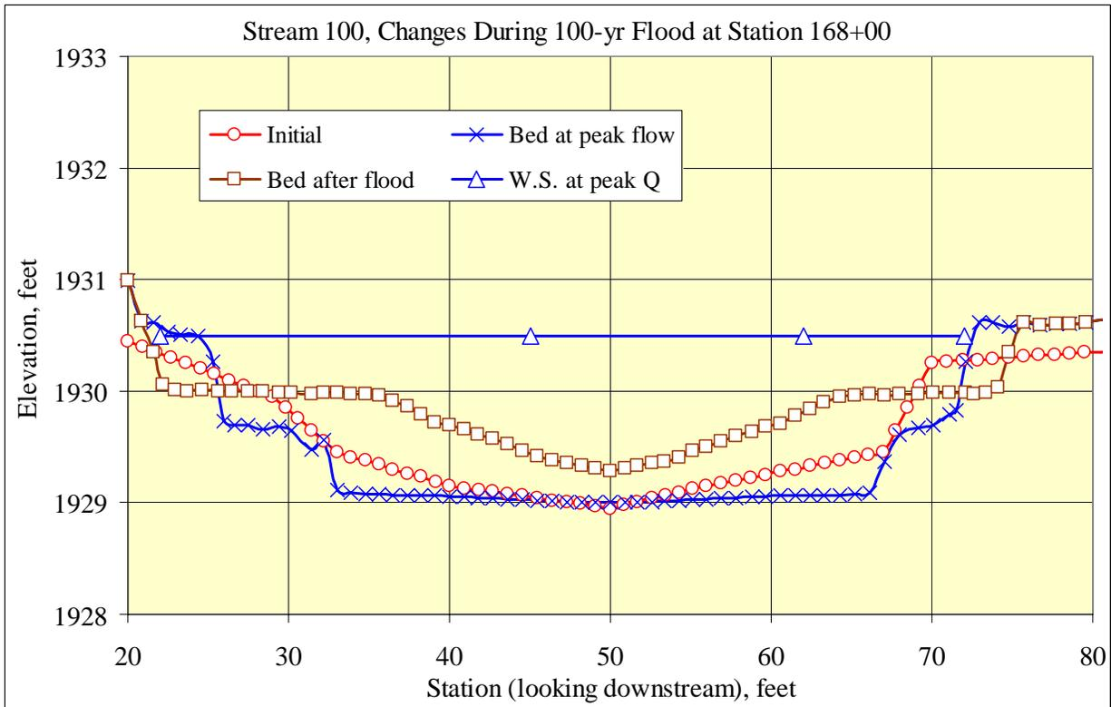
Figure 27 (continued). Simulated changes during 100-yr flood at sample cross sections along stream 100
