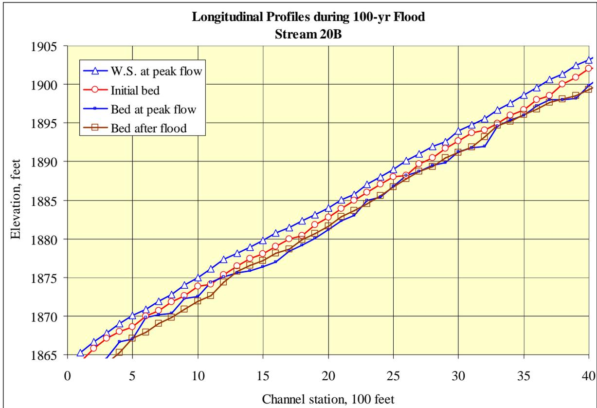
Figure 30. Water-surface and channel bed profile changes during 100-yr flood for stream 20B
