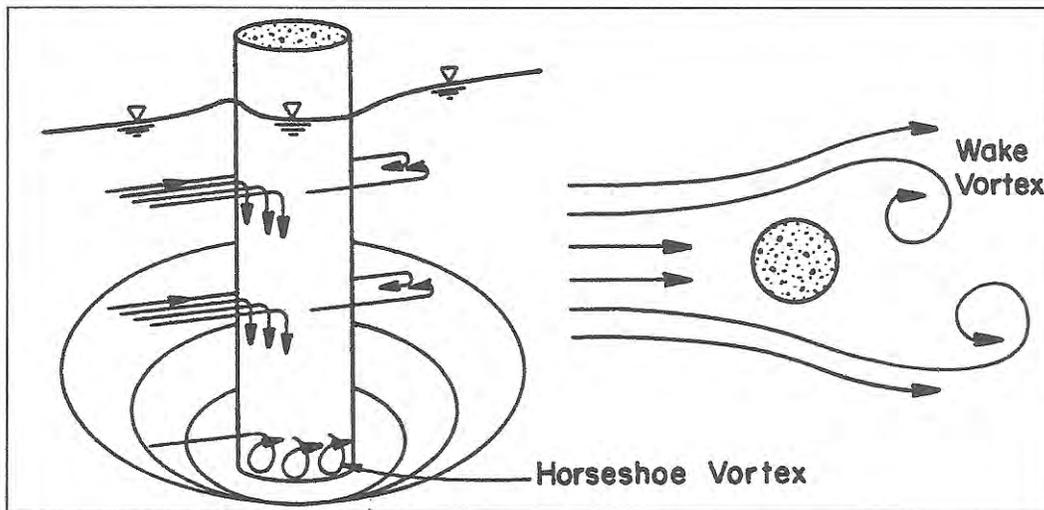
Figure 6. Interference to flow by a pier (After Federal Highway Administration, 2006)
