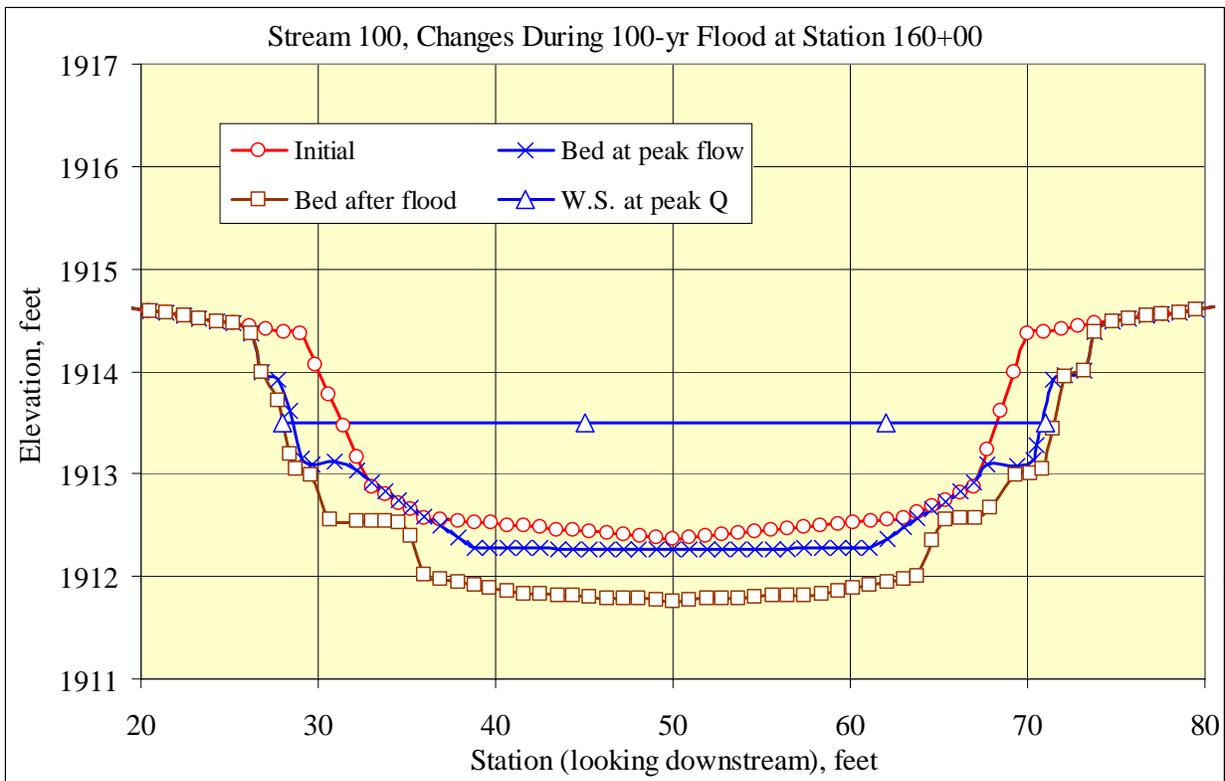
Figure 27. Simulated changes during 100-yr flood at sample cross sections along stream 100
