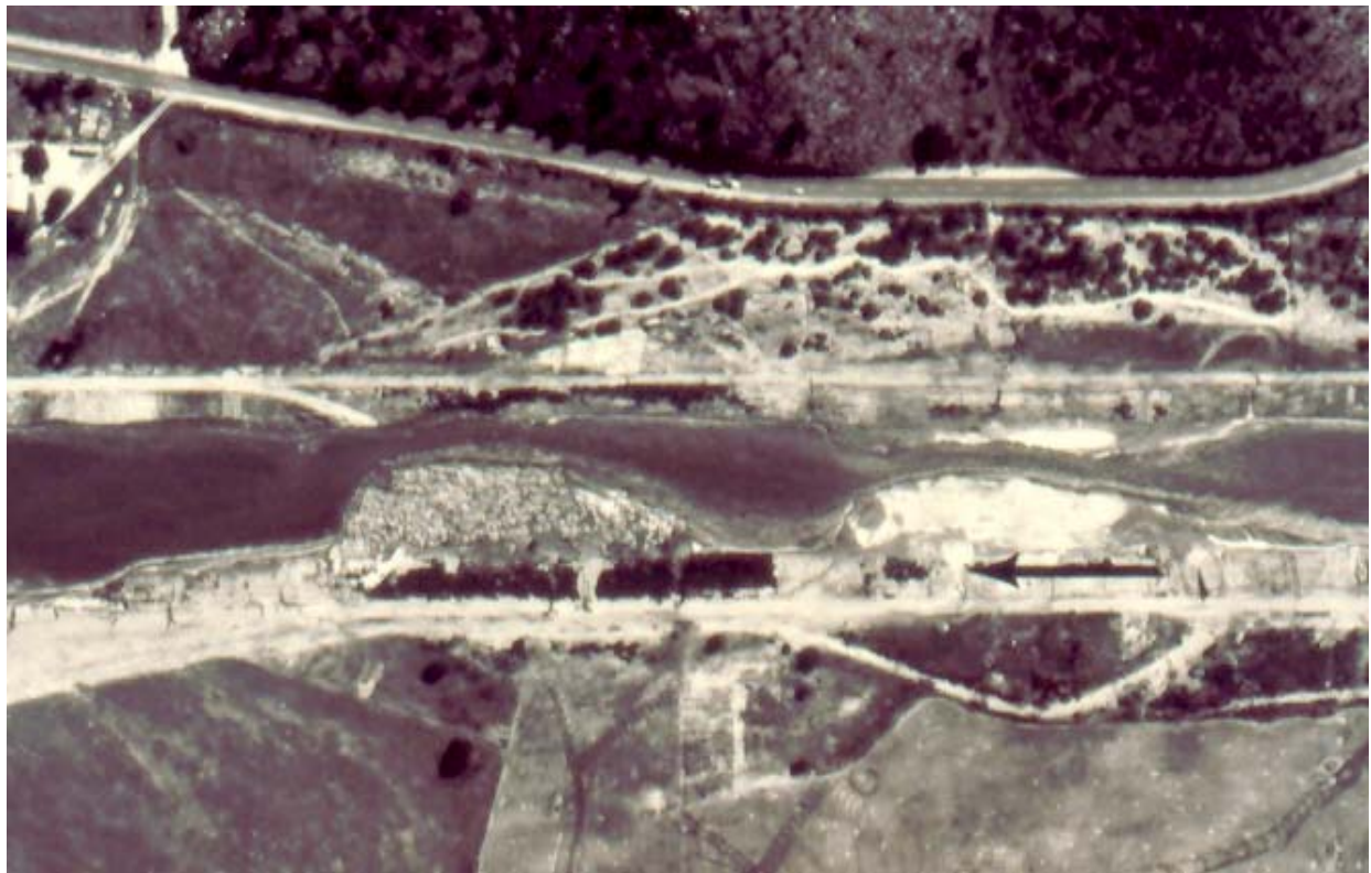
Fig. 1 Streamwise variation in width during stream channel adjustment toward establishing straight water-surface profile, San Diego River at Lakeside, California
