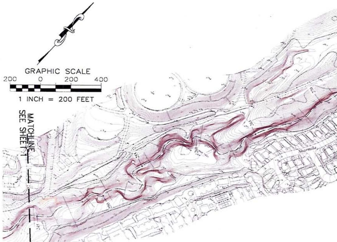
Figure 7. Topography of incised channel in Orange County, CA caused by sediment deficit
