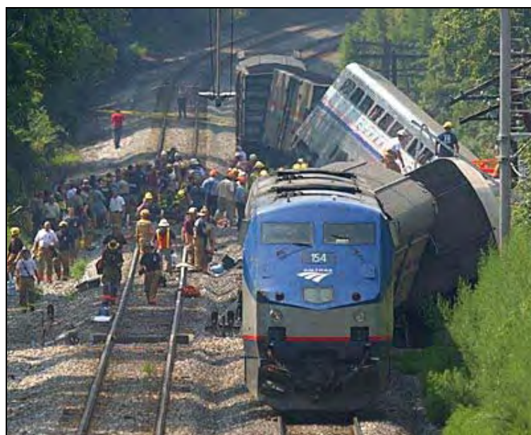
Figure 24: Trains can derail due to extreme heat warping railroad tracks.
