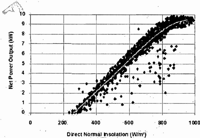
Fig. 9 SBP system net power output versus direct normal insolation
