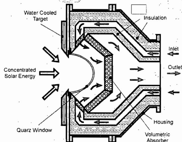
Fig. 18 DLR pressurized volumetric air receiver
