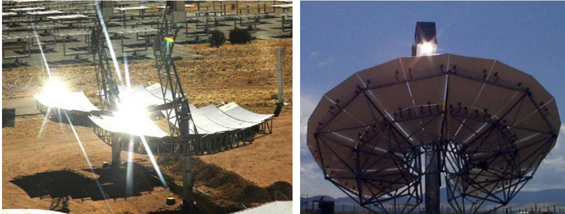
Figure 3. Left: Specular reflections from stowed parabolic dish collectors. Right: Diffuse light emanating from dish receiver aperture. (National Solar Thermal Test Facility, SNL, NM)
