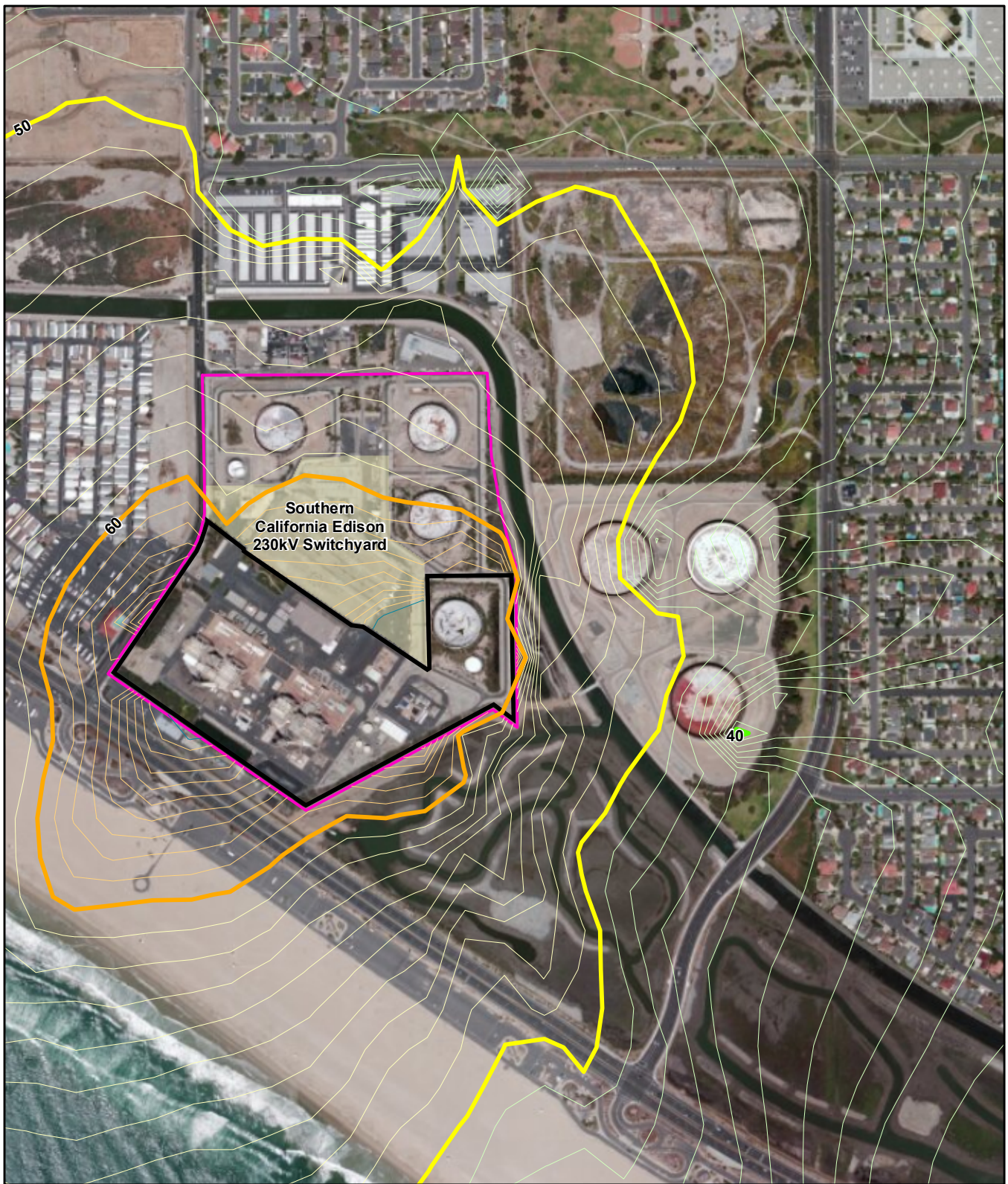
Figure DR PYLE 6-1 Estimated Sound Level Contours: Both HBEP Block 1 and Block 2 at Full Load – Facility Sound Only AES Huntington Beach Energy Project Huntington Beach, California
