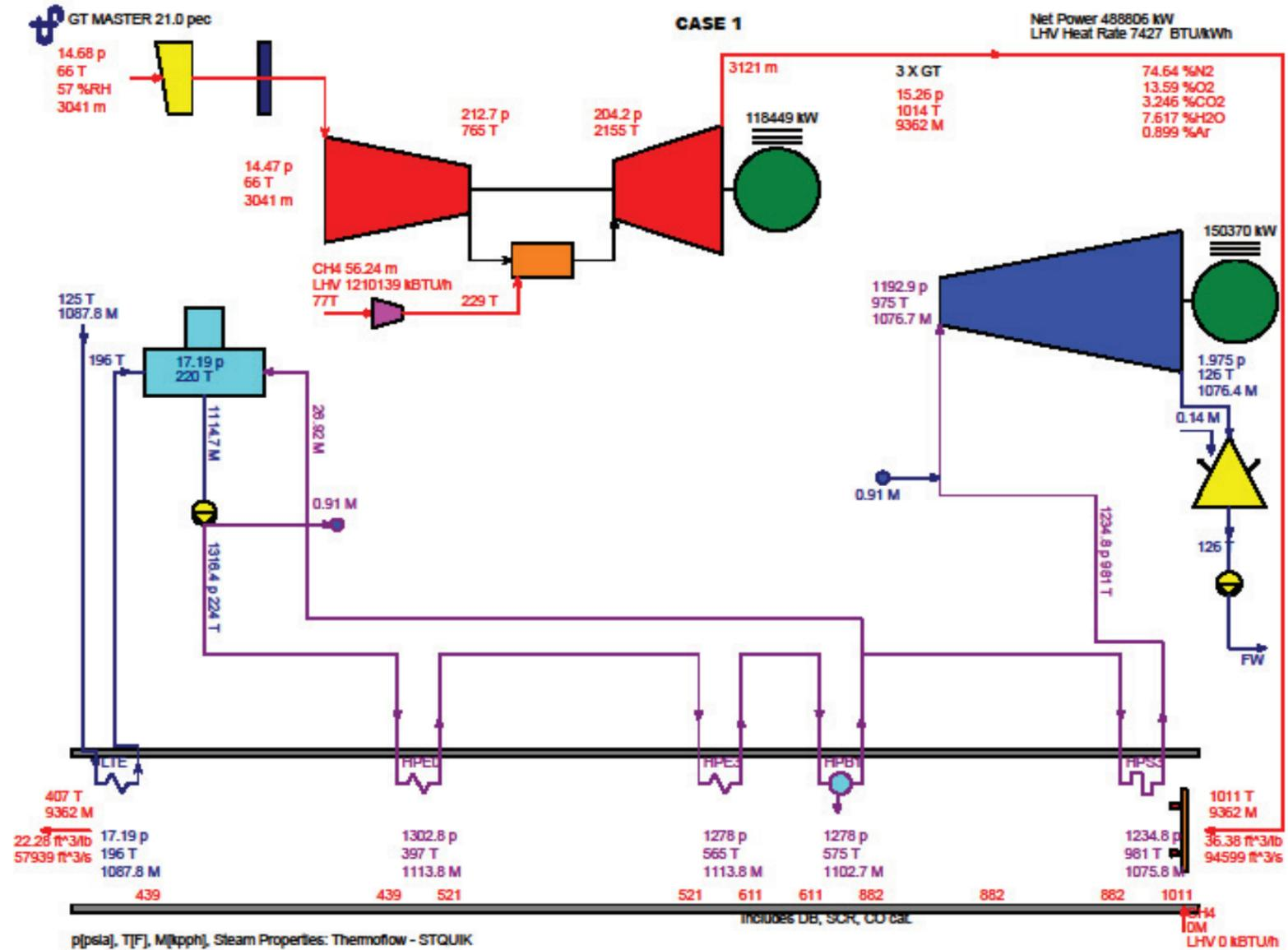
Case 1 Heat Balance Number 1a Three Combustion Turbines Operating at Maximum Heat Input without Evaporative Cooling
