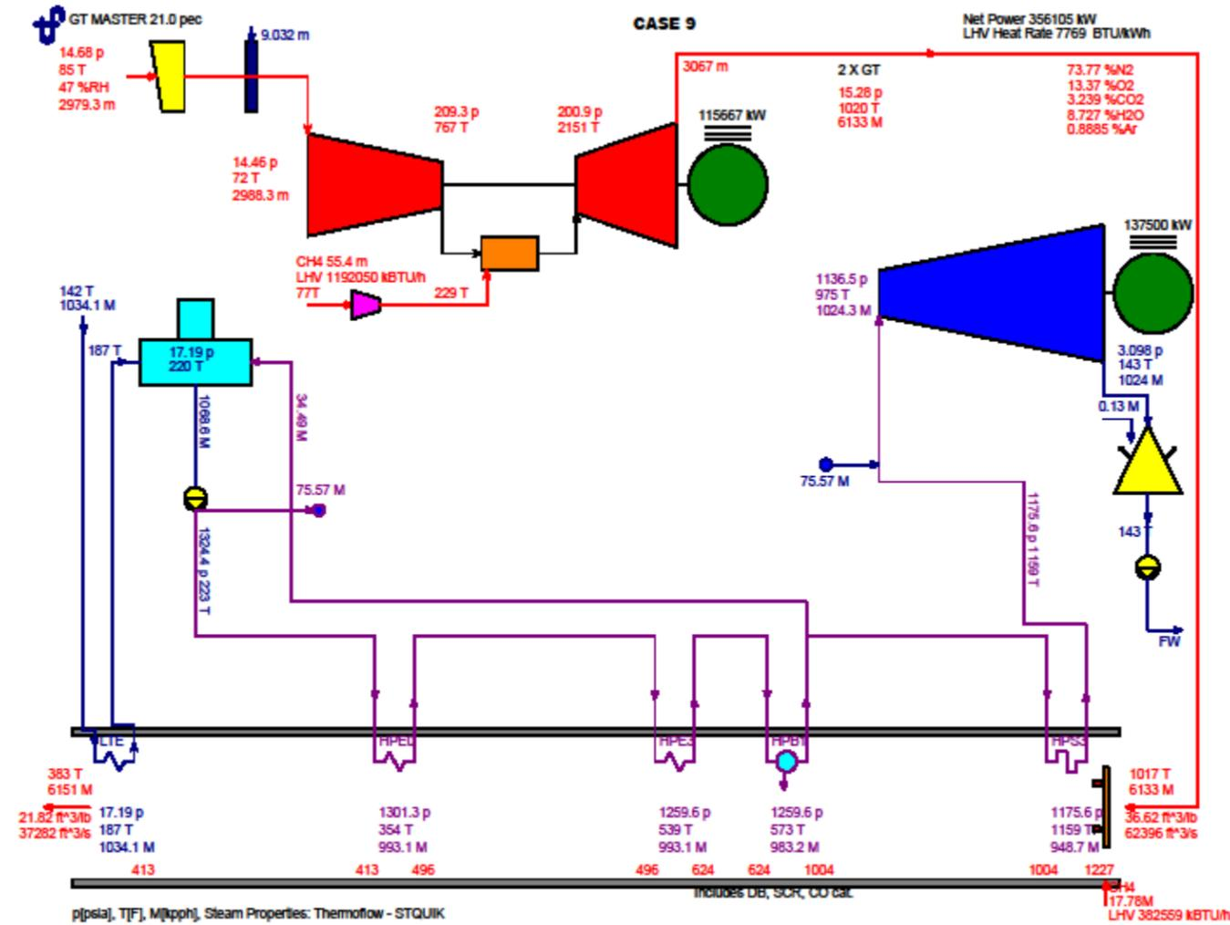
Case 9 Heat Balance Number 3b(1) Two Combustion Turbines Operating at Maximum Heat Input with Evaporative Cooling and Duct Burner
