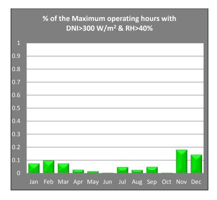
Figure DR 151-2. Percent of Maximum Operating Hours with DNI greater than 300 W/m2 and RH greater than 40 Percent.
