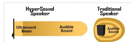
HyperSound travels in a focused direction along the beam, unlike typical point source loudspeakers that emit sound waves in all directions.
