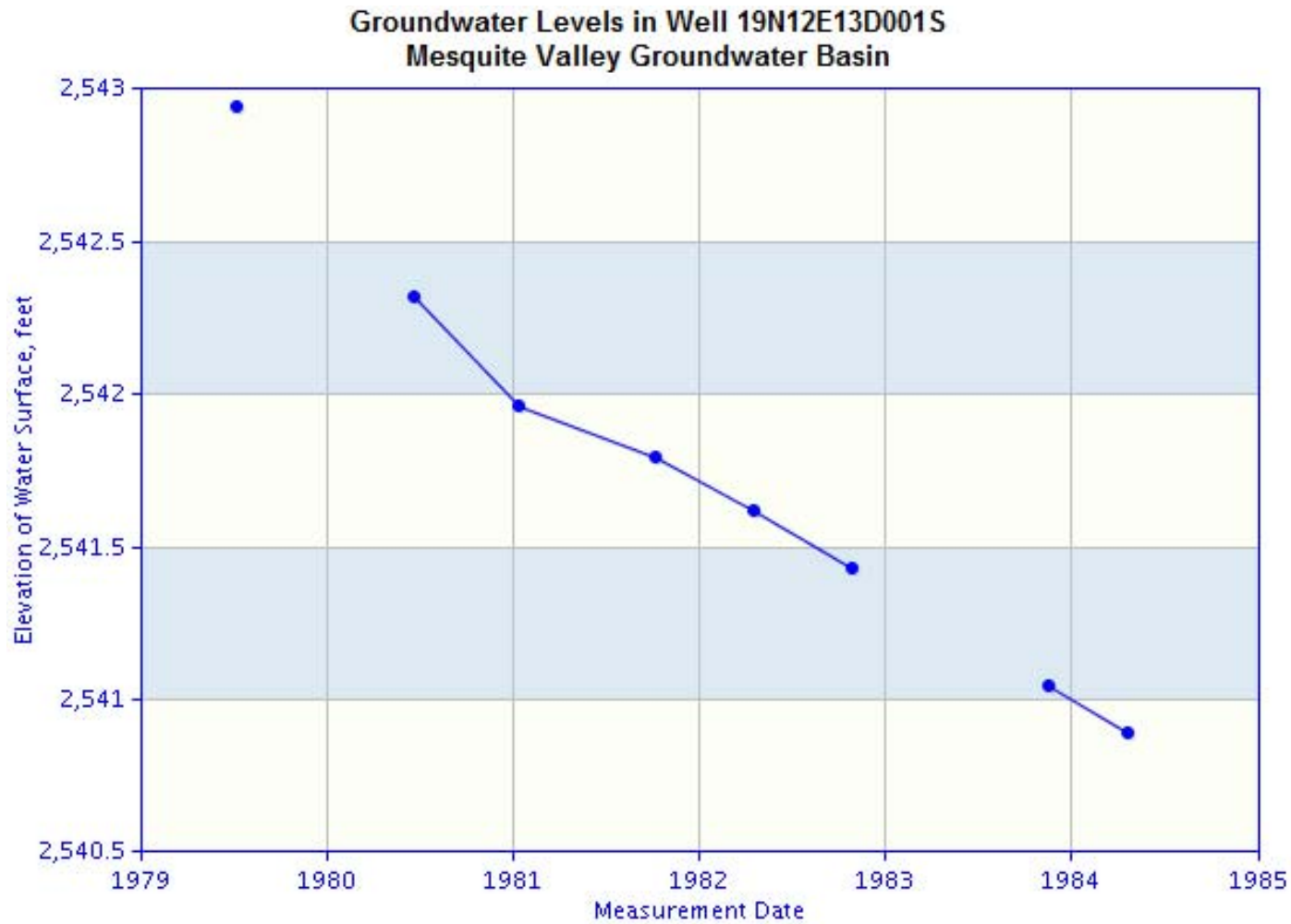
FIGURE DR137-7 Groundwater Level Decline in Vicinity of Solar Plant Alternative Solar Plant Alternative Site, Inyo County Hidden Hills Solar Electric Generating System
