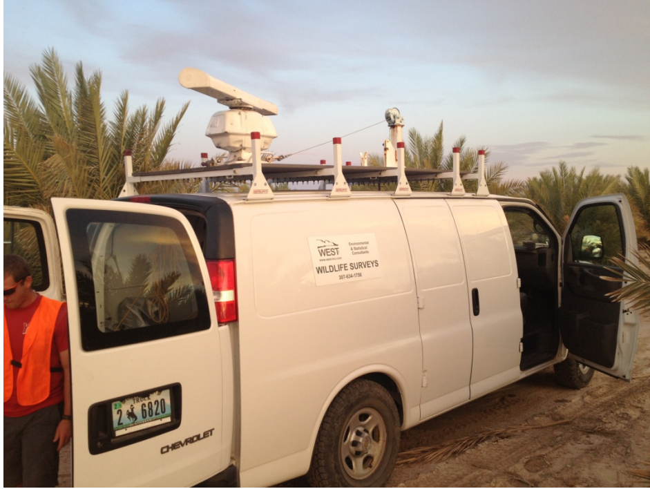
Photo A. Radar van parked at the Palen Solar Electric Generating System Radar Study Area. Antenna is in horizontal mode.
