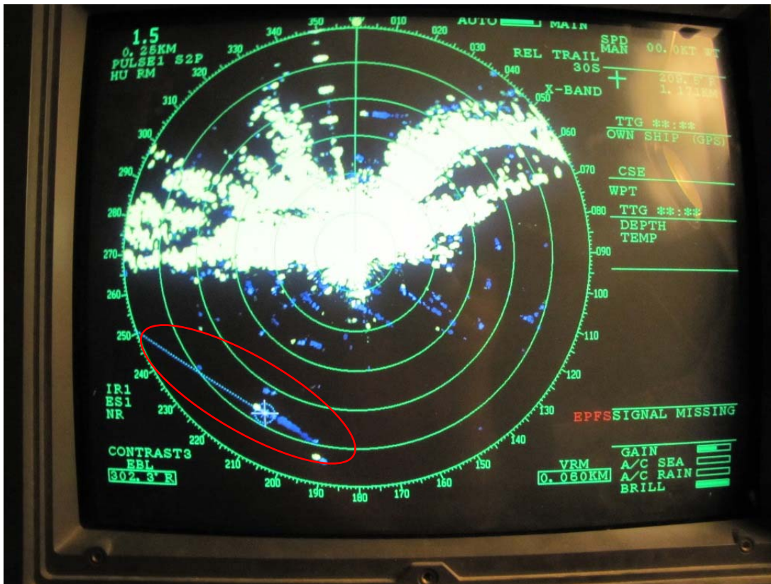
Photo E. Target speed and direction are determined in horizontal mode, establishing a bearing line and measuring distance between echo trails corresponding to speed in meters/5 seconds. The circled target was traveling 302.3° at a speed of 60 m/5 s.
