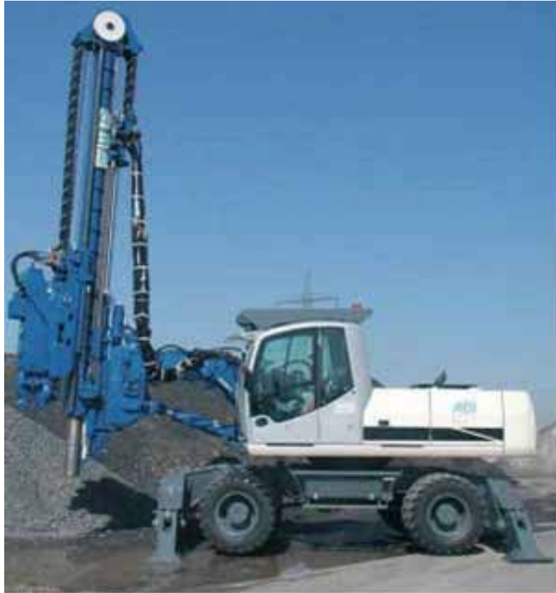
FIGURE 1-5 CONCEPTUAL PYLON DRIVING MACHINE
