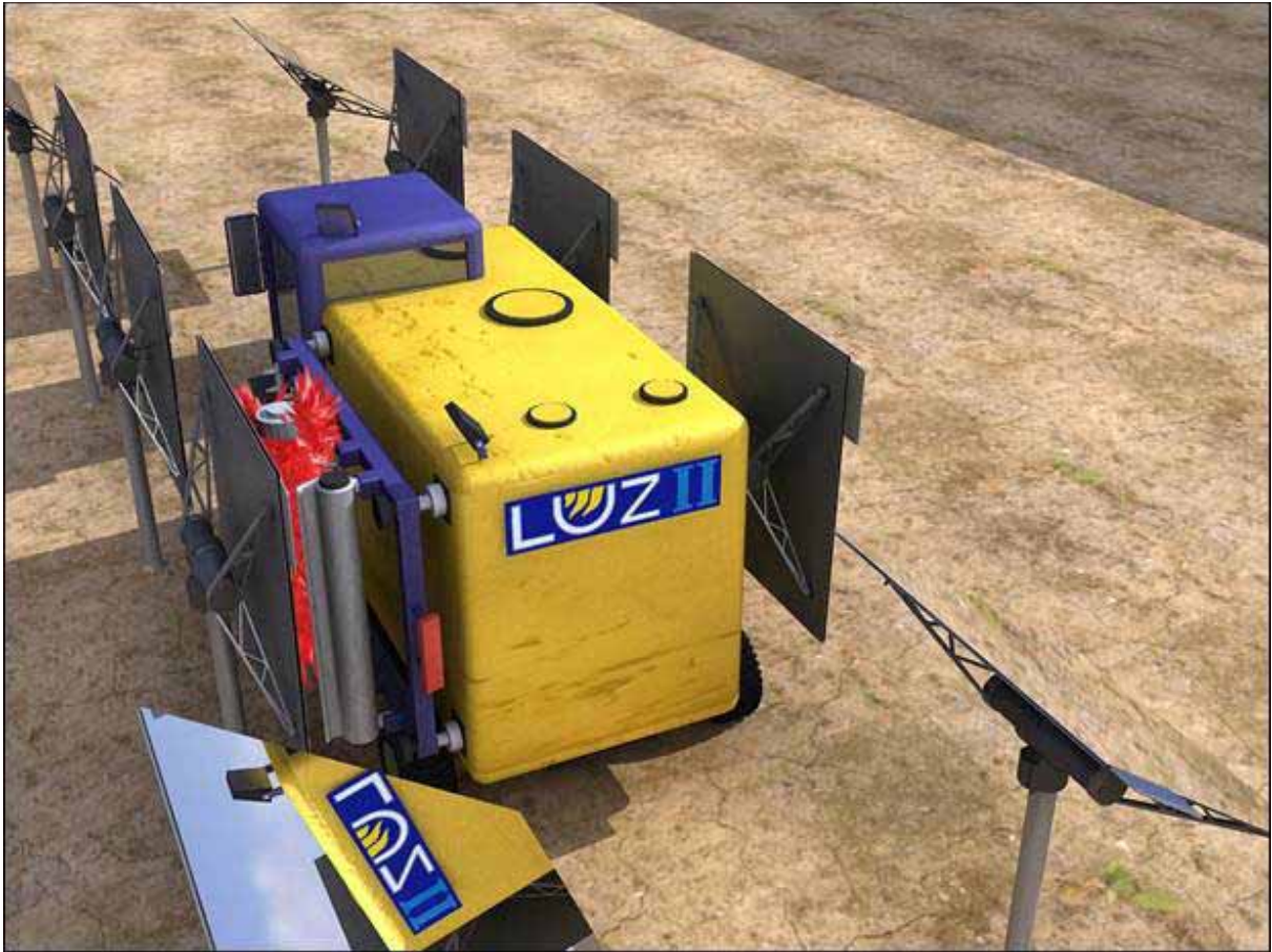
FIGURE 1-9 CONCEPTUAL MIRROR WASHING MACHINE IVANPAH SOLAR ELECTRIC GENERATING SYSTEM
