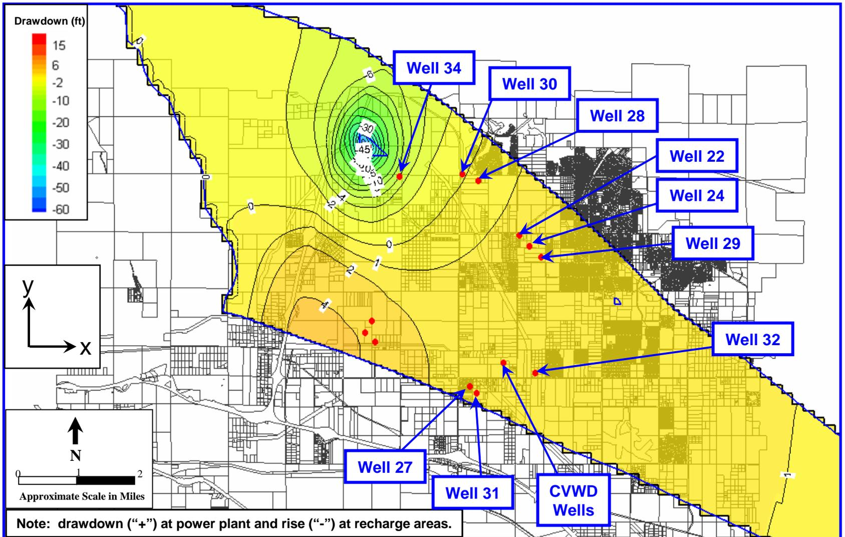
**Figure 10: Contour Map of Simulated Groundwater Level Changes at 31 Years – Scenario 2, Anisotropy Ratio =2
