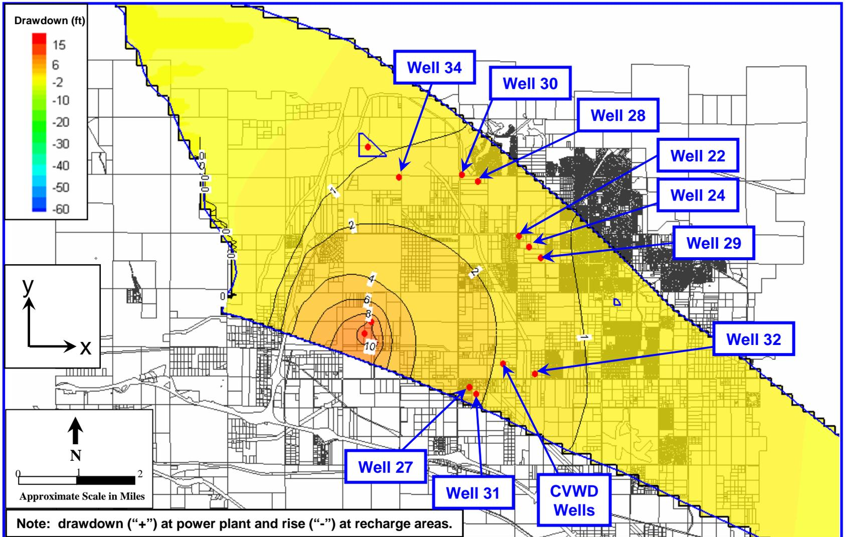
**Figure 6: Contour Map of Simulated Groundwater Level Changes at 5 Years – Scenario 2, Anisotropy Ratio =1
