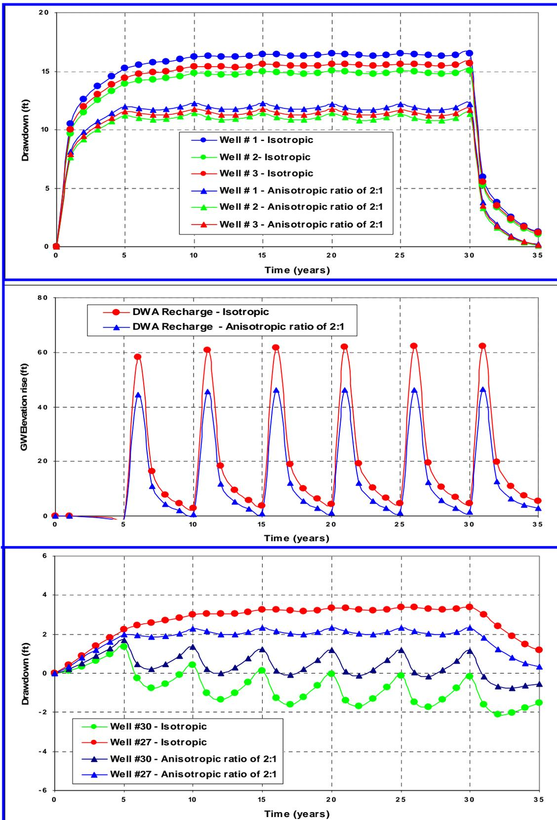
Figure 12: Scenario 2 Results at Project Pumping Wells, DWA Recharge Basin and MSWD Wells 27 and 30 (Pumping = 1,100 afy, Recharge = 5,500 afy every 5 years)
