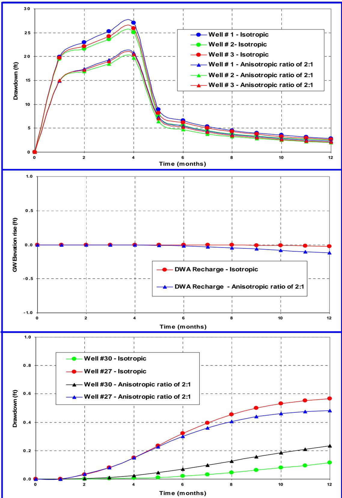
Figure 17: Scenario 3 Results at Project Pumping Wells, DWA Recharge Basin and MSWD Wells 27 and 30 (Pumping = 2,059 gpm, No recharge, Total pumping volume = 1,100 af)
