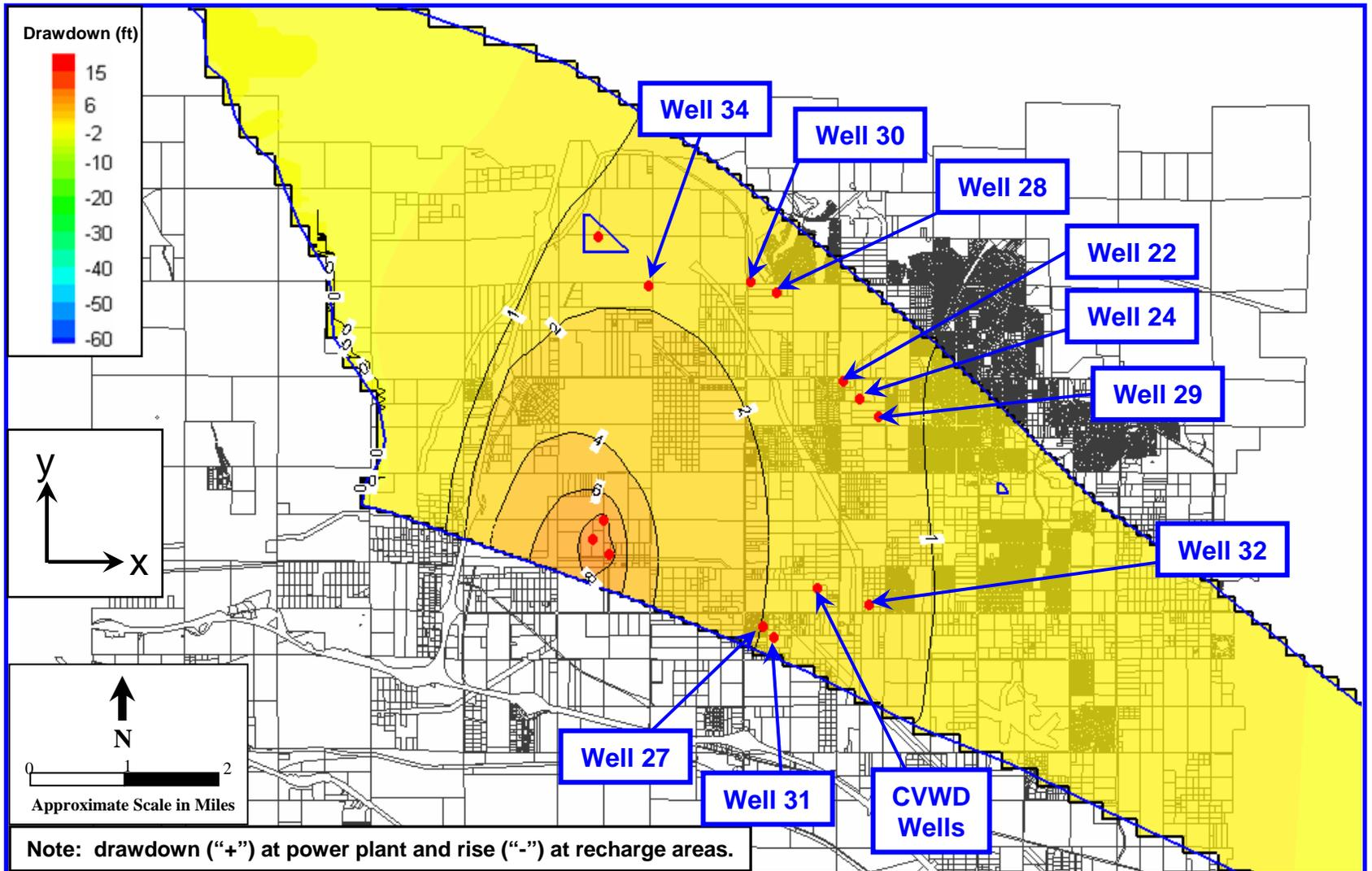
**Figure 9: Contour Map of Simulated Groundwater Level Changes at 5 Years – Scenario 2, Anisotropy Ratio =2
