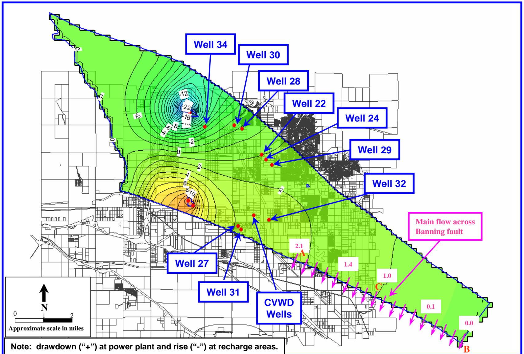
**Figure 5: Contour Map of Simulated Groundwater Level Changes at 30 Years – Scenario 1, Anisotropy Ratio =1**
