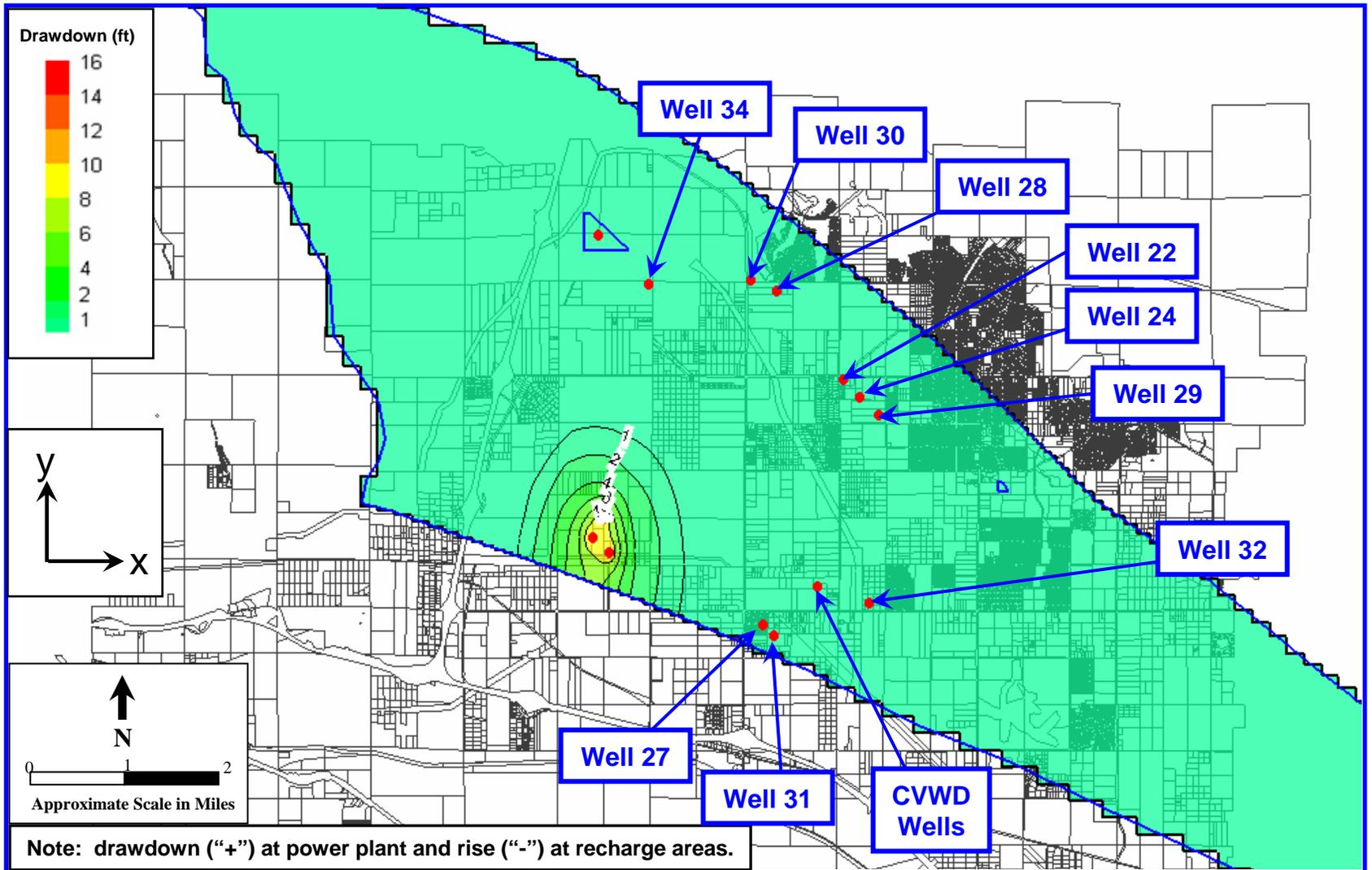
**Figure 15: Contour Map of Simulated Groundwater Level Changes at 4 Months – Scenario 3, Anisotropy Ratio =2
