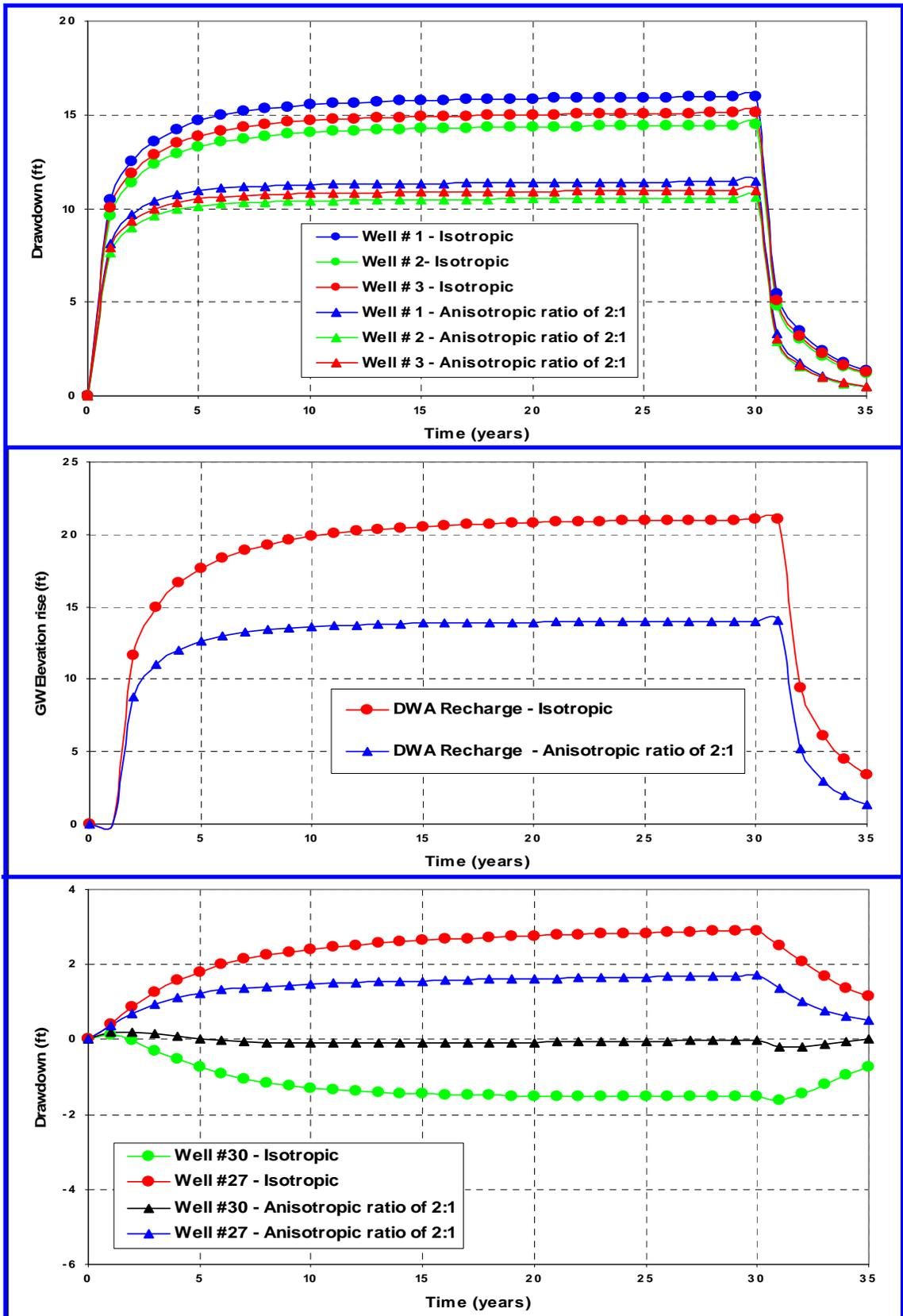
Figure 5: Scenario 1 Results at Project Pumping Wells, DWA Recharge Basin and MSWD Wells 27 and 30 (Pumping = 1,100 afy, Recharge = 1,100 afy)
