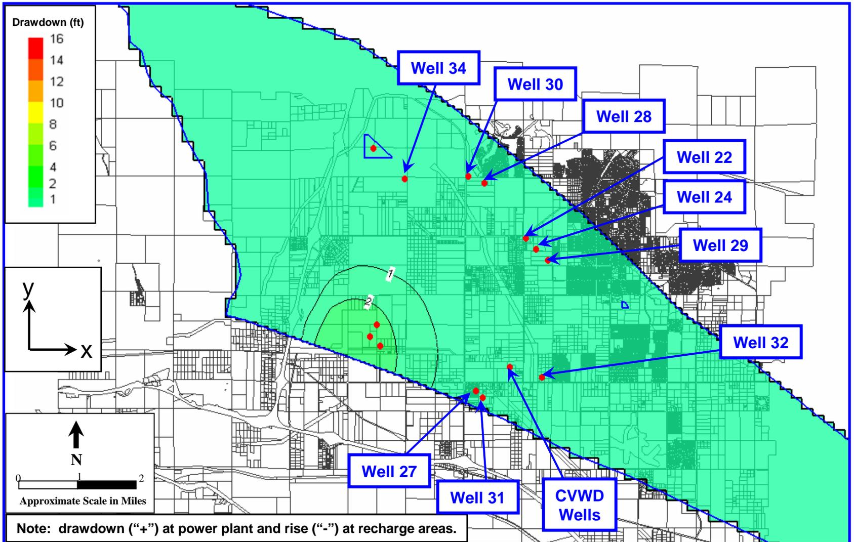
**Figure 14: Contour Map of Simulated Groundwater Level Changes at 12 Months – Scenario 3, Anisotropy Ratio =1
