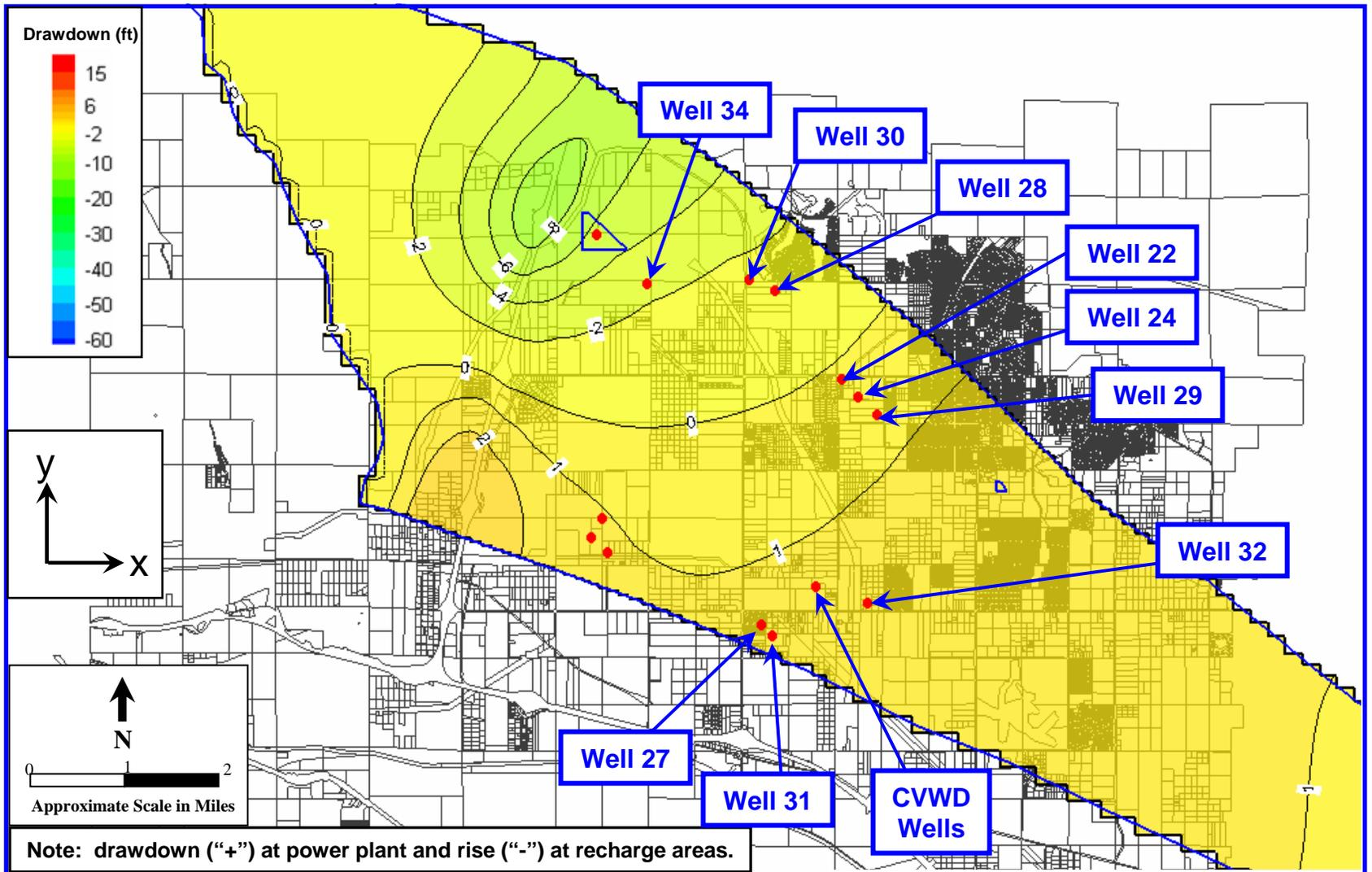
**Figure 8: Contour Map of Simulated Groundwater Level Changes at 35 Years – Scenario 2, Anisotropy Ratio =1
