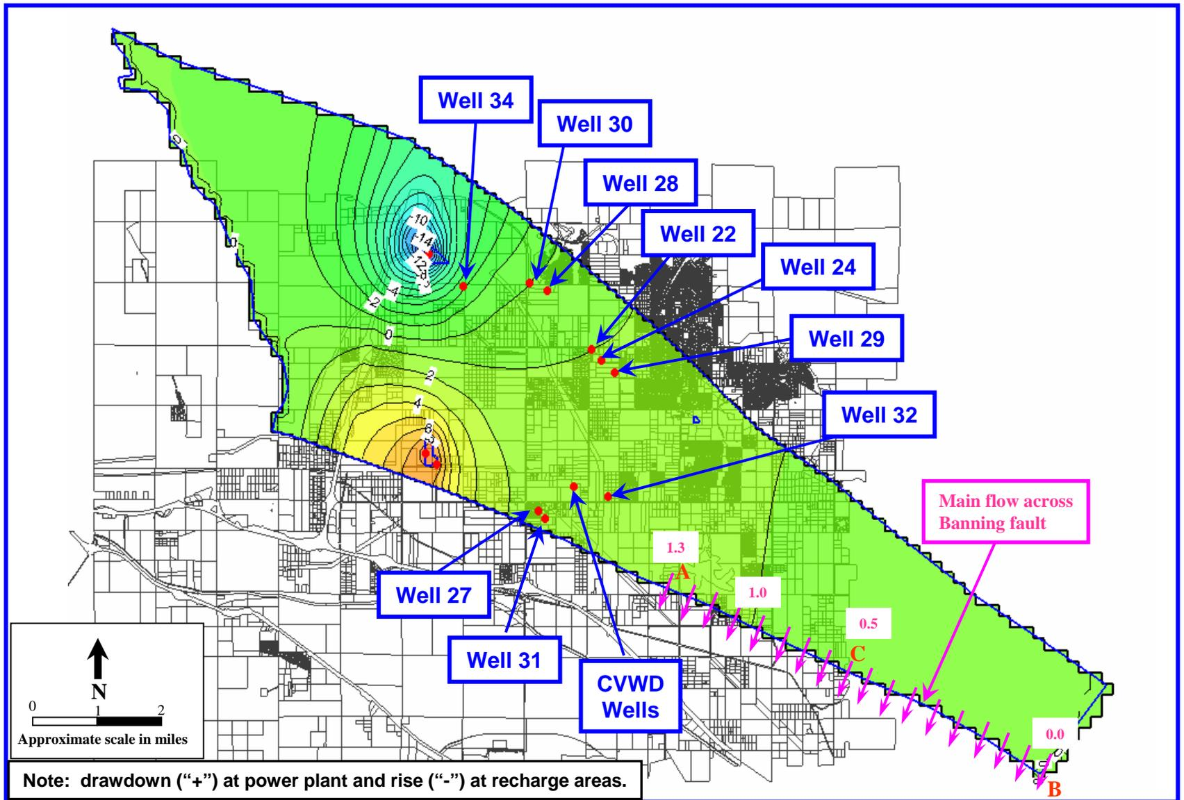
**Figure 4: Contour Map of Simulated Groundwater Level Changes at 30 Years – Scenario 1, Anisotropy Ratio =2
