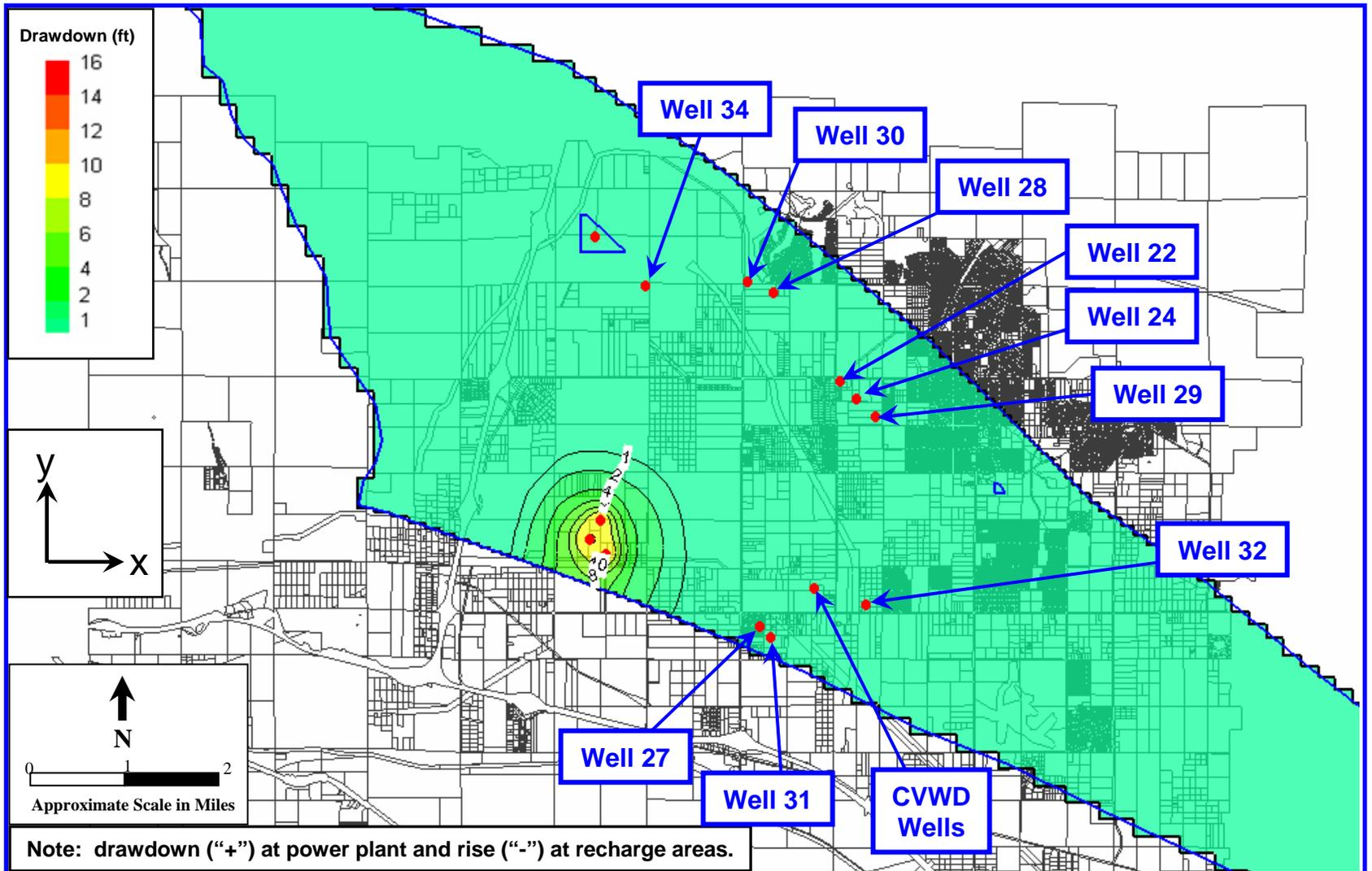
**Figure 13: Contour Map of Simulated Groundwater Level Changes at 4 Months – Scenario 3, Anisotropy Ratio =1
