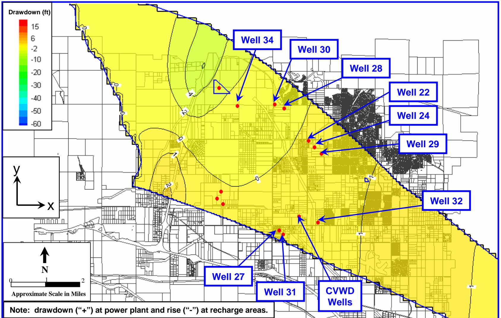
**Figure 11: Contour Map of Simulated Groundwater Level Changes at 35 Years – Scenario 2, Anisotropy Ratio =2
