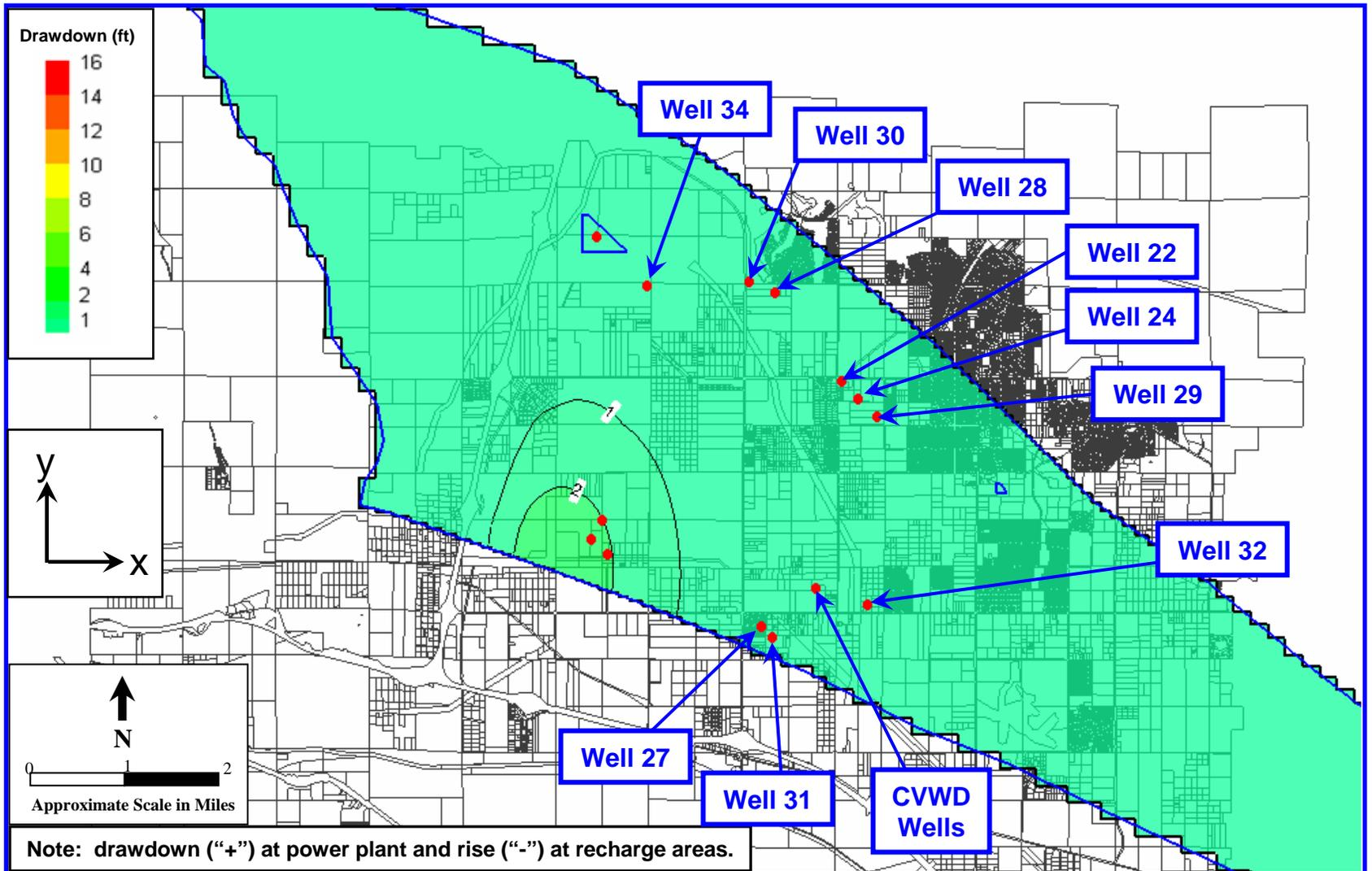
**Figure 16: Contour Map of Simulated Groundwater Level Changes at 12 Months – Scenario 3, Anisotropy Ratio =2
