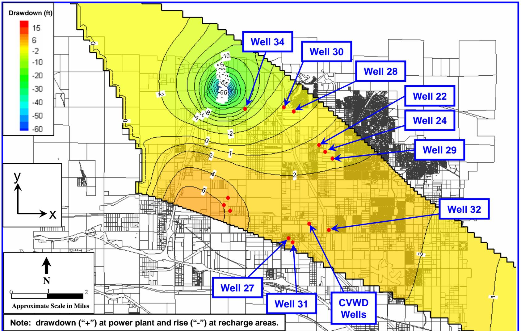
**Figure 7: Contour Map of Simulated Groundwater Level Changes at 31 Years – Scenario 2, Anisotropy Ratio =1
