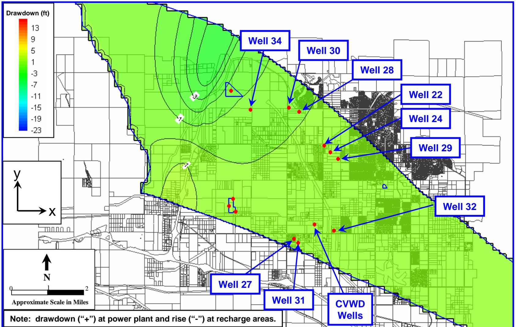
**Figure 4: Contour Map of Simulated Groundwater Level Changes at 35 Years – Scenario 1, Anisotropy Ratio =2
