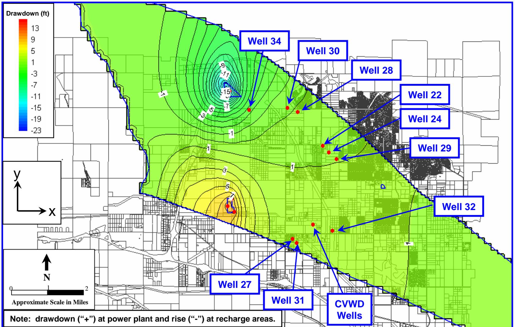
**Figure 3: Contour Map of Simulated Groundwater Level Changes at 30 Years – Scenario 1, Anisotropy Ratio =2
