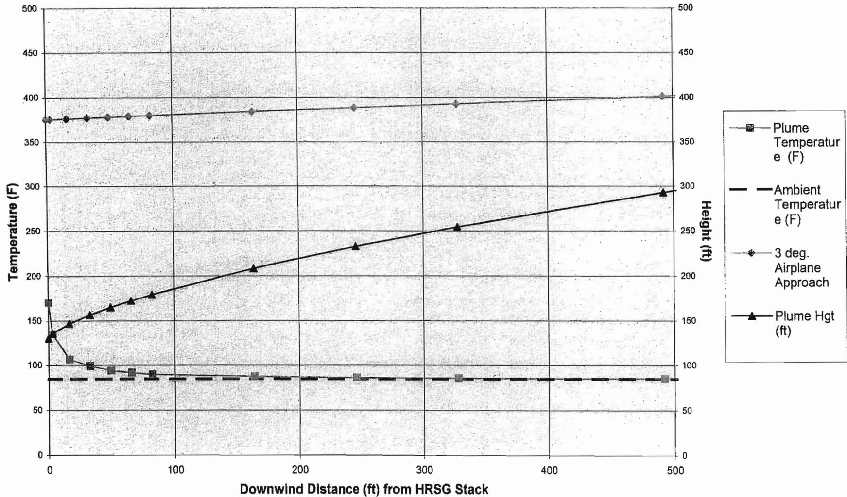
Figure 5. HRSG- Plume Temperature and Height (Detail)
