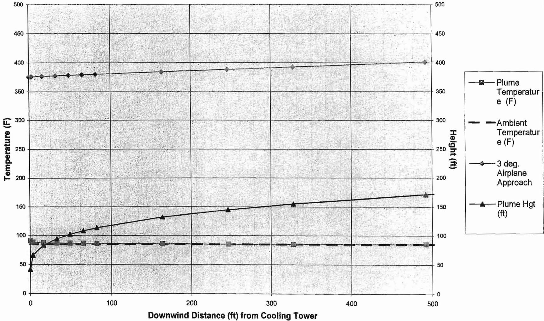
**Figure 11. Cooling Tower- Plume Temperature and Height (Detail)**
