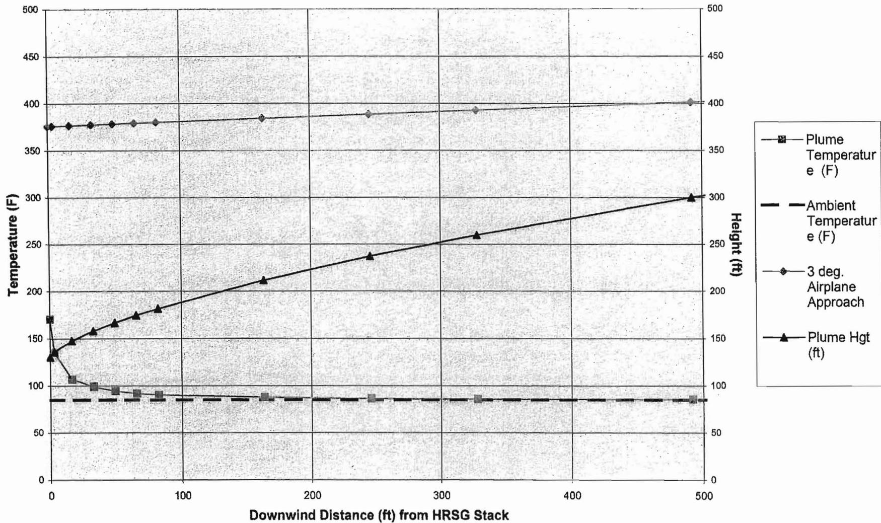
Figure 4. HRSG- Plume Temperature and Height (Detail)
