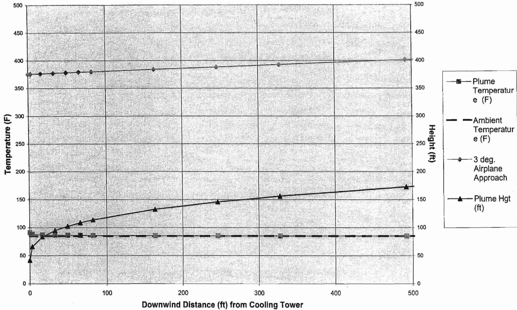
**Figure 10. Cooling Tower- Plume Temperature and Height (Detail)
