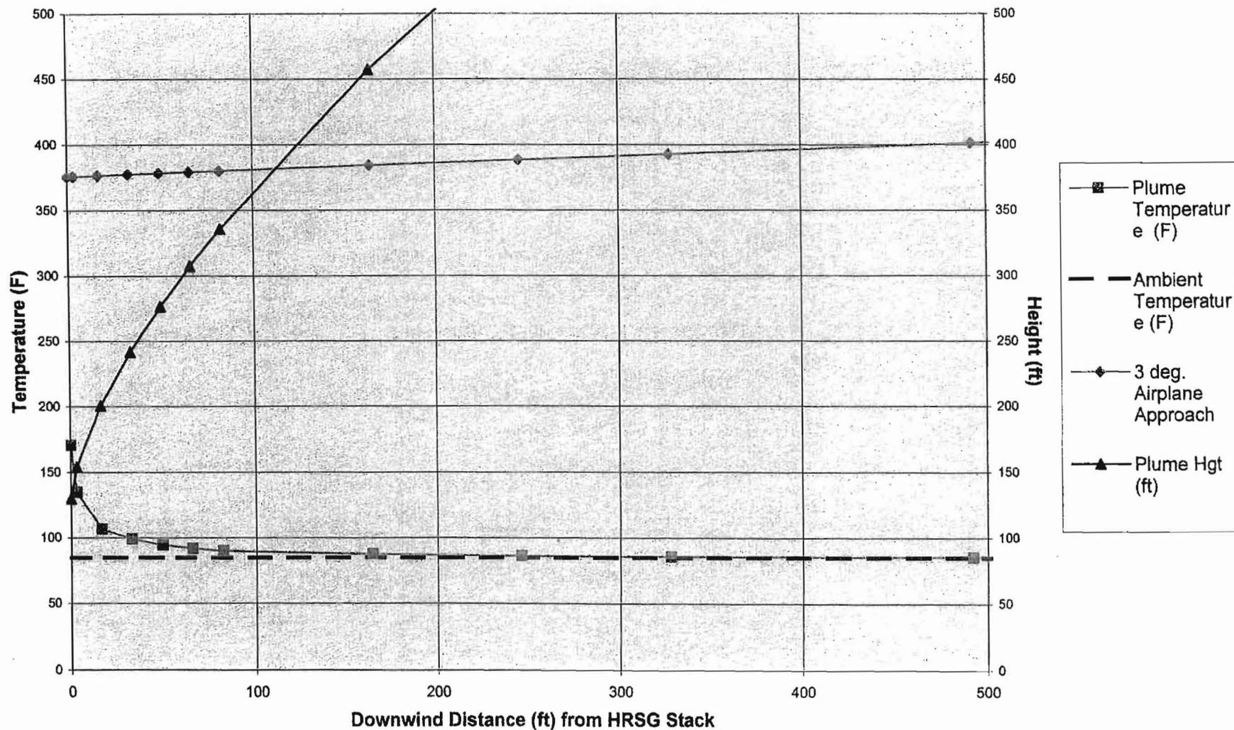
**Figure 2. HRSG- Plume Temperature and Height (Detail)
