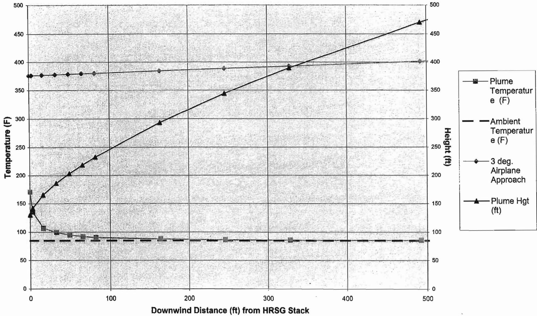
**Figure 3. HRSG- Plume Temperature and Height (Detail)
