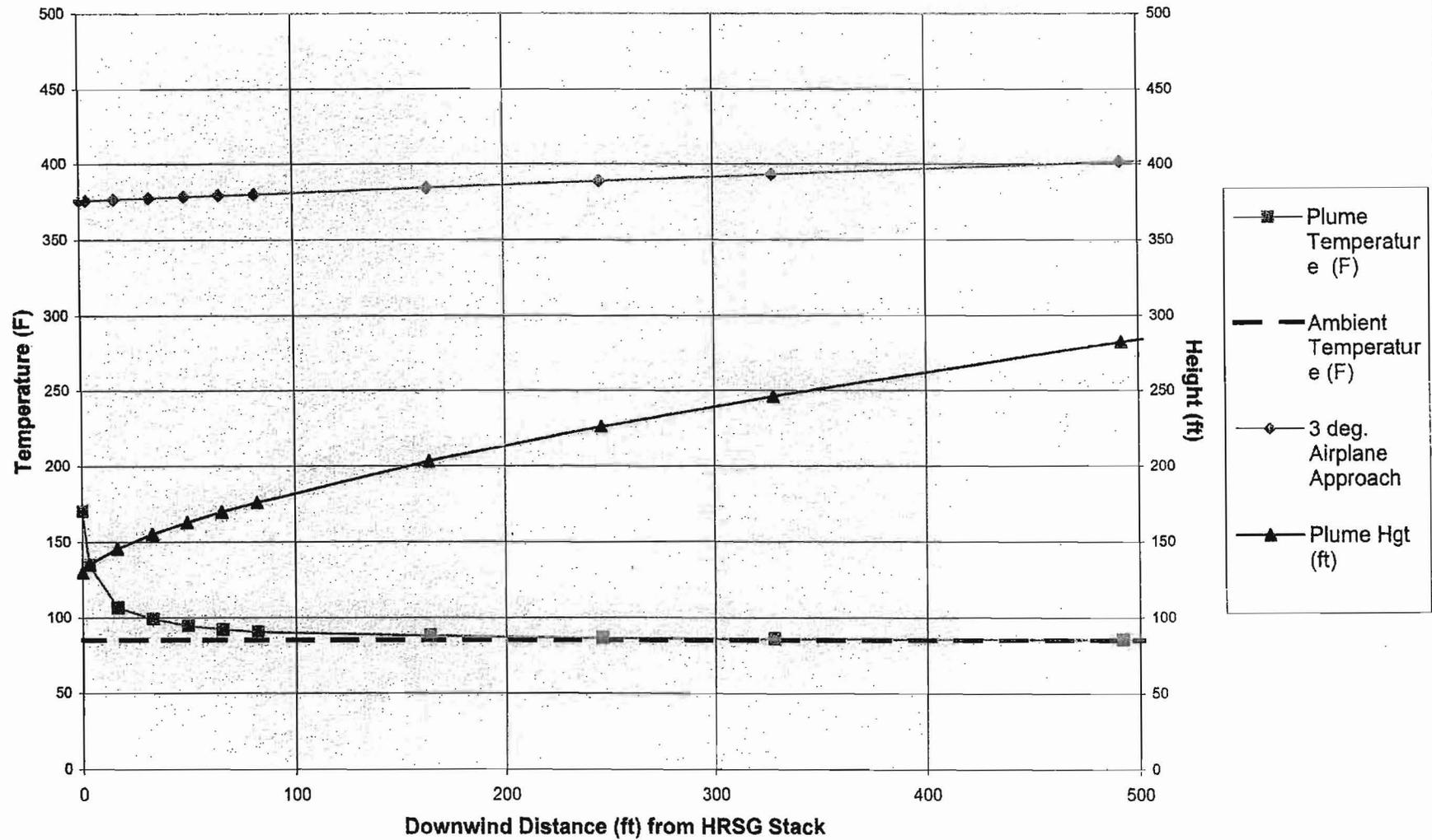
**Figure 7. Cooling Tower- Plume Temperature and Height (Detail)**
