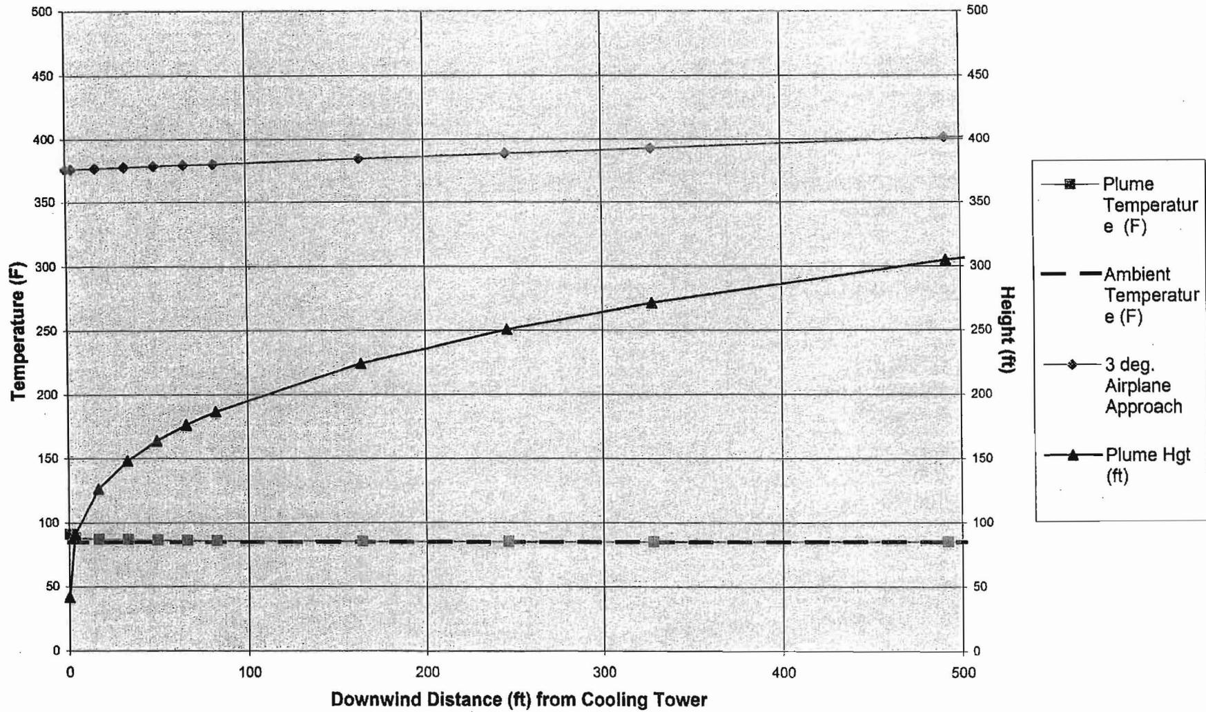
**Figure 9. Cooling Tower- Plume Temperature and Height (Detail)
