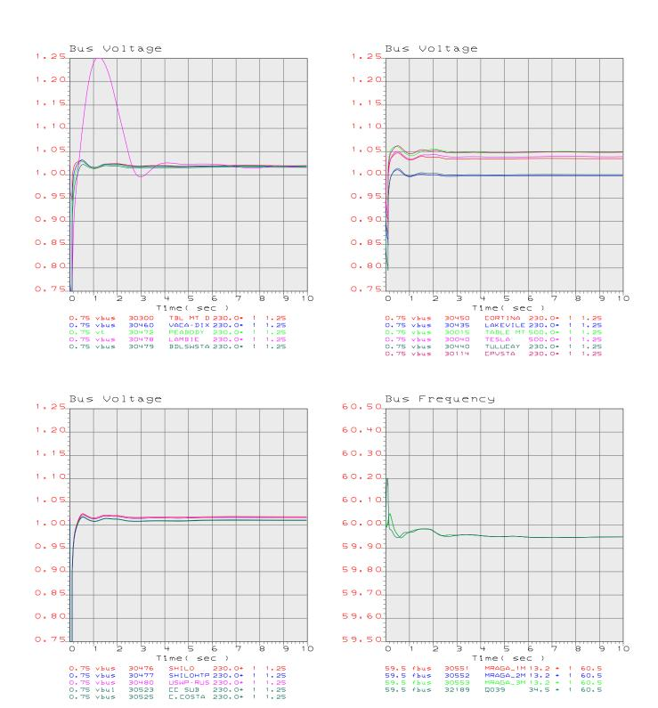
PG8E 2007 CASE SERIES: 2013 Greater Bay Area Summer Peak Post-Project Case PATH15=-1714 MW(S-N) PATH26= 3933 MW(N-S) PDEI= 2500 MW(N-S) COI= 4731 MW(N-S) Q275 630 MW at Vaca-Dixon-Lambie8Peabody IFS - 2013 Summer Peak Post-Project FY Lambie - Q275SWST and Lambie - Birds 230 kV Double Line Out
