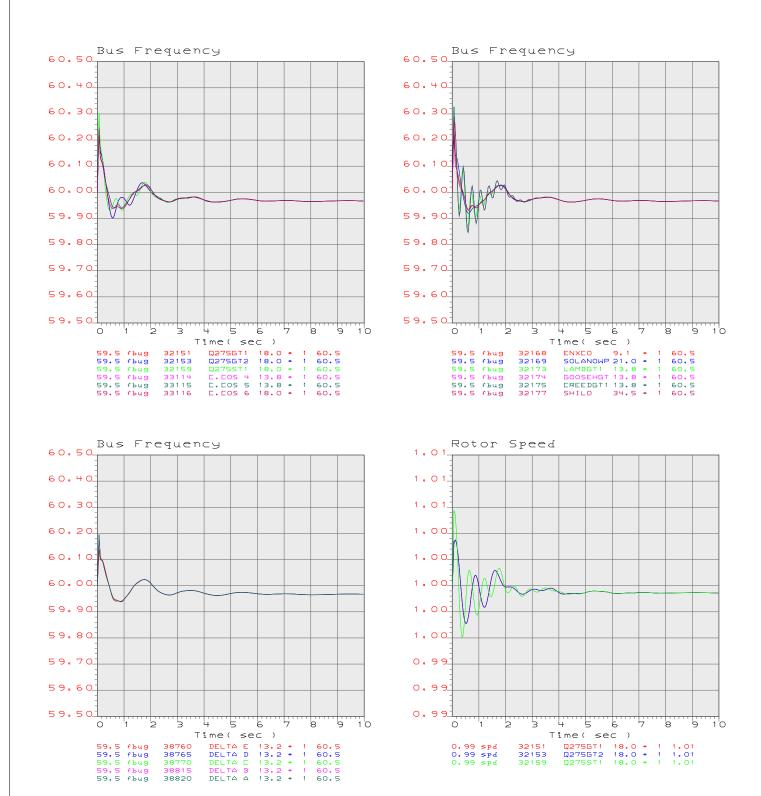
PG8E 2007 CASE SERIES: 2013 Greater Bay Area Summer Peak Post-Project Case PATH15=-1714 MW(S-N) PATH26= 3933 MW(N-S) PDEI= 2500 MW(N-S) COI= 4731 MW(N-S) Q275 630 MW at Vaca-Dixon-Lambie8Peabody IFS - 2013 Summer Peak Post-Project FY Table Mt - Tesla and Vaca-Dixon - Tesla 500-kV Double Line Out
