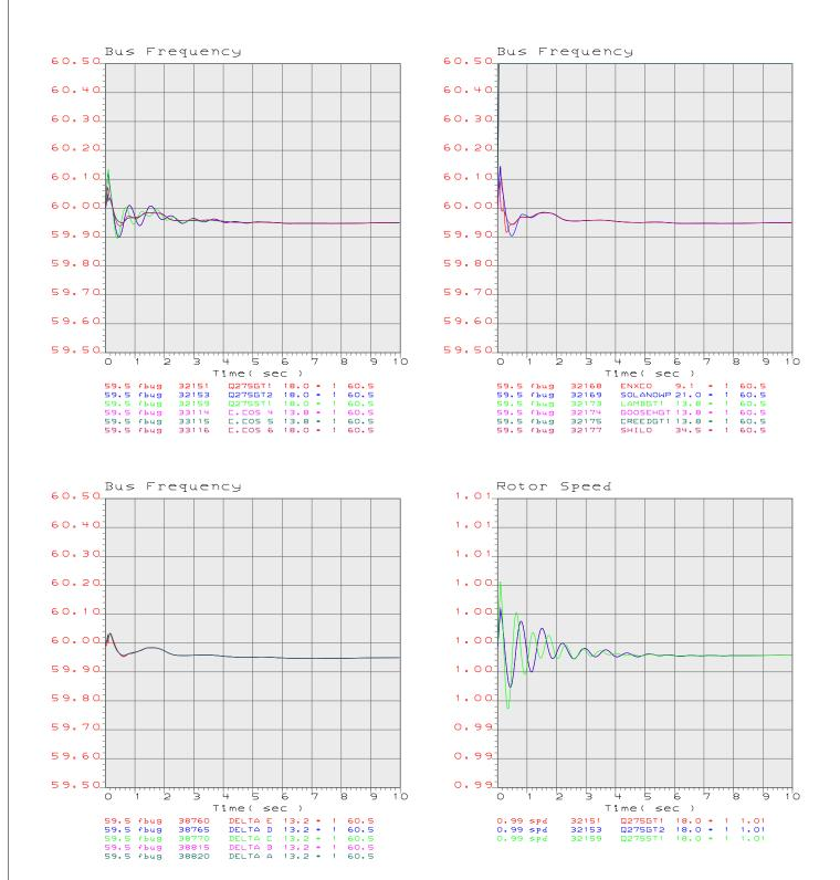
PG8E 2007 CASE SERIES: 2013 Greater Bay Area Summer Peak Post-Project Case PATH15=-1714 MW(S-N) PATH26= 3933 MW(N-S) PDCI= 2500 MW(N-S) COI= 4731 MW(N-S) Q275 630 MW at Vaca-Dixon-Lambie8Peabody IFS - 2013 Summer Peak Post-Project FY Lambie - Q275SWST and Lambie - Birds 230 kV Double Line Out
