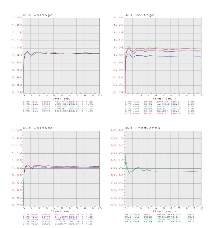
PG8E 2007 CASE SERIES: 2013 Greater Bay Area Summer Peak Post-Project Case PATH15=-1714 MW(S-N) PATH26= 3933 MW(N-S) PDEI= 2500 MW(N-S) COI= 4731 MW(N-S) Q275 630 MW at Vaca-Dixon-Lambie8Peabody IFS - 2013 Summer Peak Post-Project FY Vaca Dixon - Table Mt and Vaca Dixon 500/230 kV Tx 500-kV Double Line Ou
