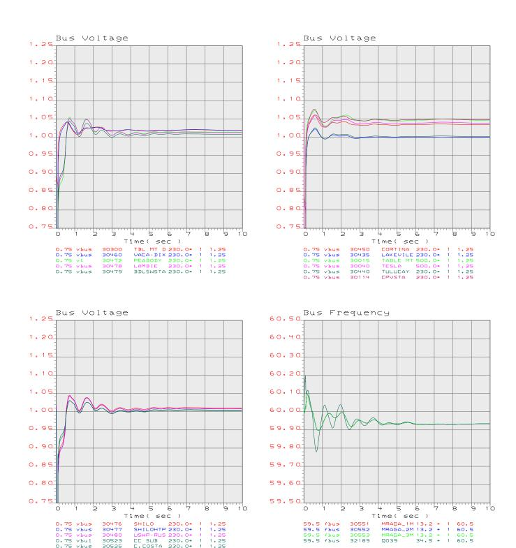
PG8E 2007 CASE SERIES: 2013 Greater Bay Area Summer Peak Post-Project Case PATH15=-1714 MW(S-N) PATH26= 3933 MW(N-S) PDEI= 2500 MW(N-S) COI= 4731 MW(N-S) Q275 630 MW at Vaca-Dixon-Lambie8Peabody IFS - 2013 Summer Peak Post-Project FY Vaca - Q275SWST #182 230 kV Double Line Out
