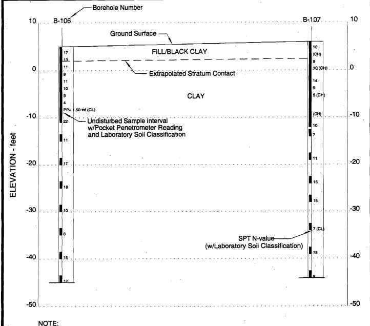
Subsurface data have been obtained only at the actual borehole locations. The stratification shown between the boreholes is based on extrapolation of the data obtained from the boreholes. Actual stratification between the boreholes may differ from that shown.
